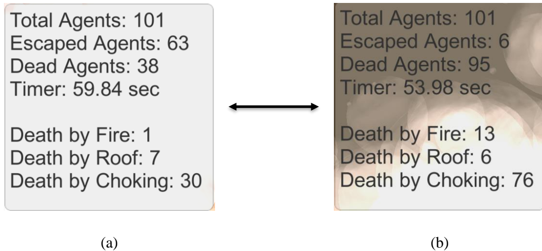
Figure 36: Comparison of (a) results of simulation using extra staff with (b) results of scenario 2
