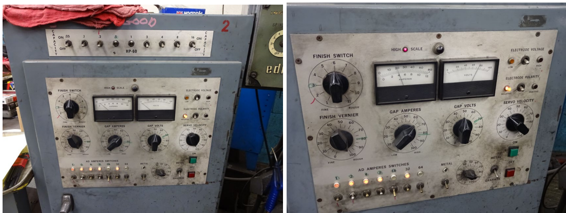
Figure 3.6. Power Generator and controls for the EDM machine
