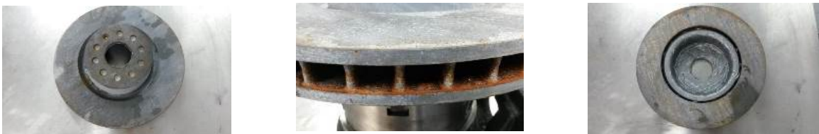
Figure 7.6. Post ASTM B117 Corrosion test pictures on processed part # 1
