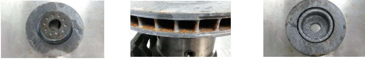
Figure 7.6. Post ASTM B117 Corrosion test pictures on processed part # 1
