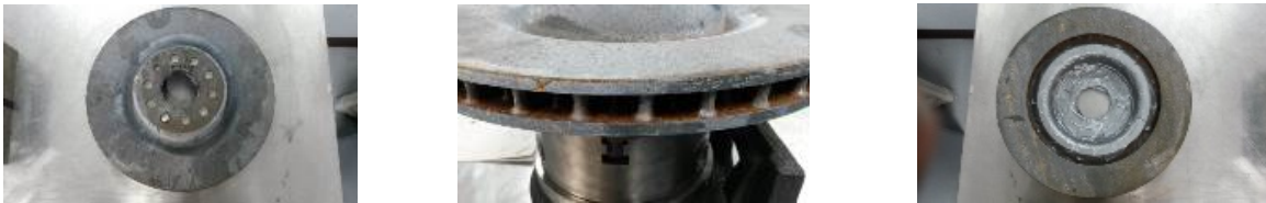
Figure 7.8. Post ASTM B117 Corrosion test pictures on processed part # 3
