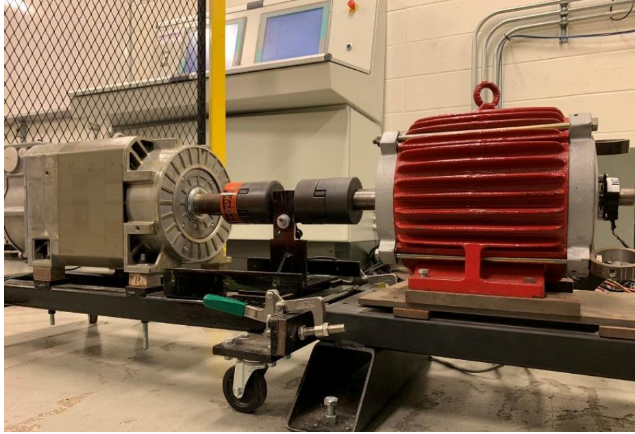
Figure 5.7. Thermal Test Setup for 4.3 kW IPMSM.
