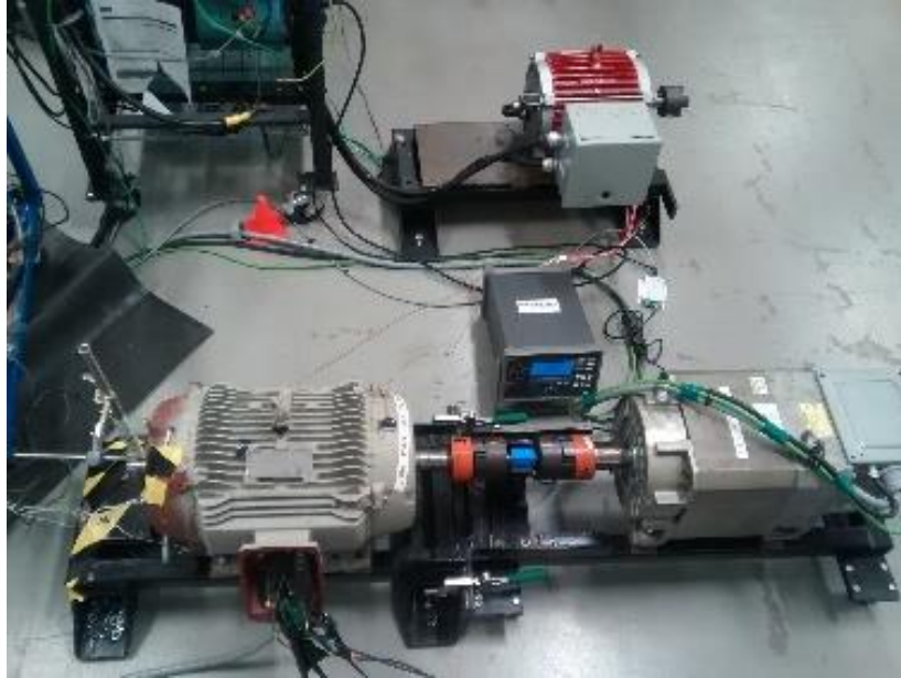
(a) DC thermal test setup.
