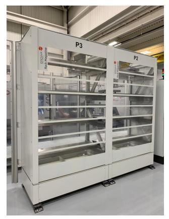
Figure 4.9 EROWA® Rack magazine
