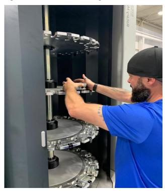
*Figure 4.11 SPM* Automation Inc. operator loading EROWA<sup>®</sup> rotary magazine
