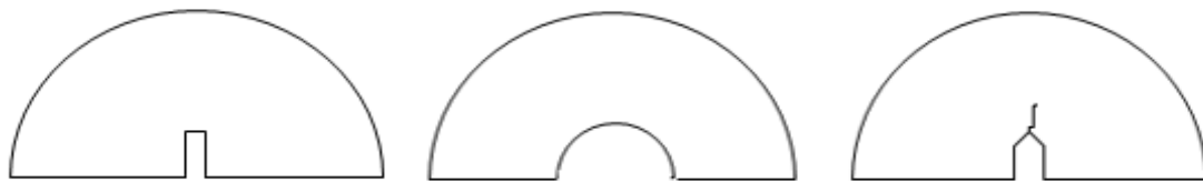
a) Rectangular notch b) Semi-Circular notch c) Fatigue Pre-cracked notch
