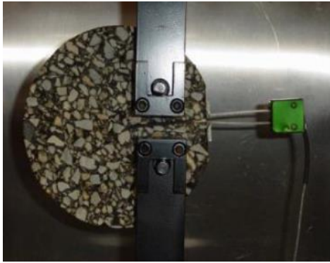
c) Disk-Shaped Compaction Test (Braham et al. , 2016)
