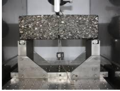
a) Single Notched Beam (Braham et al. , 2016)
