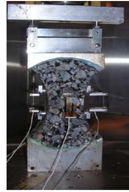
d) Dog-Bone Direct Tension (Koh et al. , 2009)
