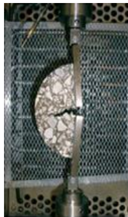
Figure 1.5 Fénix Test Setup (Perez-Jimenez et al., 2010)
