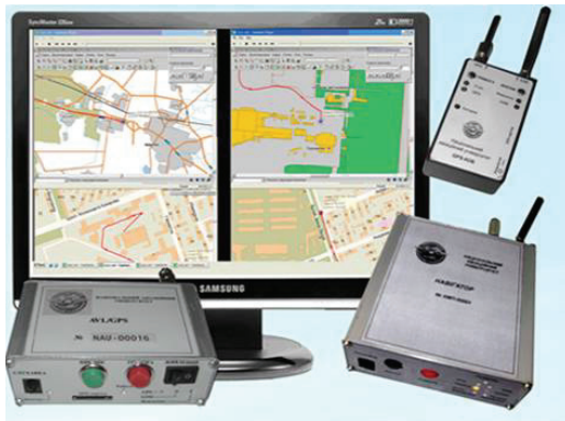
Figure 13 – Hardware-software complex for special moving vehicles monitoring and control
