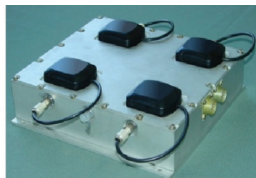
Figure 6 – The prototype of 4-element adaptive antenna array
