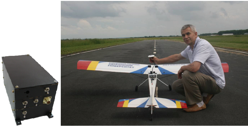
Figure 14 – Small UAV used for the experimental testing of GNSS/INS navigation system prototype
