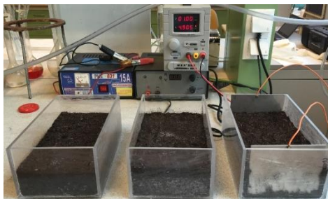
Fig. 1. Experimental setup (from left to right: control box with soil without bacteria; box with bacteria; box with bacteria under influence of electric current)
