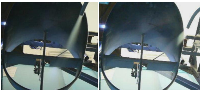
Fig 8 - CPW model in wind tunnel T-5, airflow V=35 m/sec. Smoke visualization
