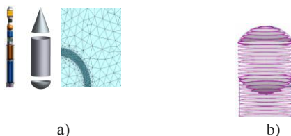
Fig.1. Elements of casing constructions (a) and scheme of construction breakdown to the ring finite elements (b)
