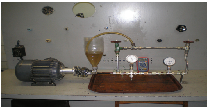
Fig. 1. General scheme of experimental fluidizer for liquids research
