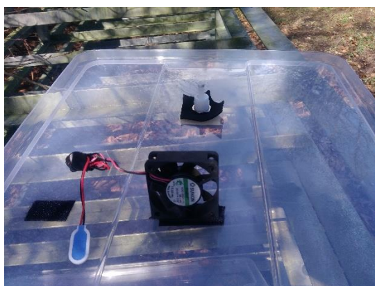
Figure 3.4 Lid used for air measurements with a fan in Scotland
