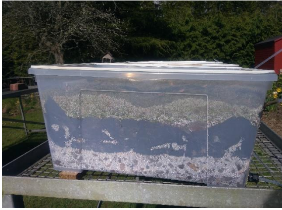
Figure 3.2 Boxes assembled in Scotland for treatment with soil and garden waste (left) and with soil and no garden waste (right)
