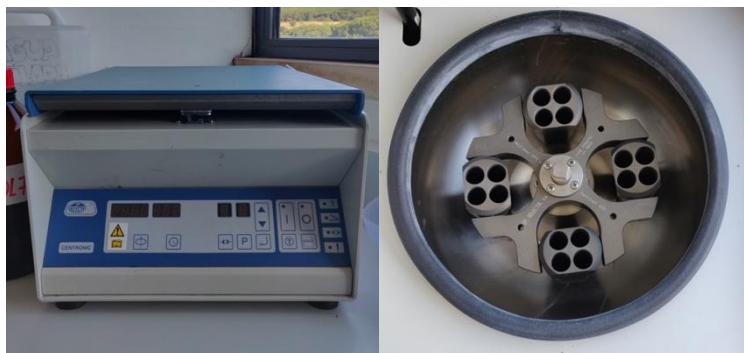
Figure 23 – Centromix II-BL centrifuge used in CIISA's laboratory, with a rotating motor of 7 cm of radii (Original).
