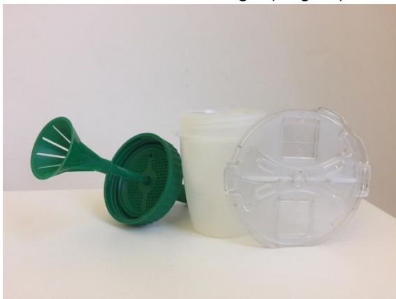
Figure 221 – Fill-FLOTAC with its container, sampling kit and built in filter and the reading disk, Mini-FLOTAC, on the right (Original).
