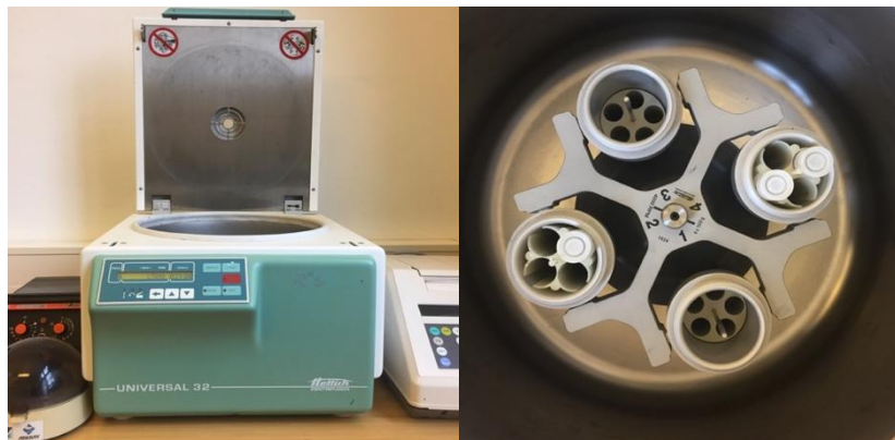
Figure 20 – Hettich Universal 32 centrifuge used in ARTIS' laboratory, with a rotating motor of 7 cm of radii (Original).
