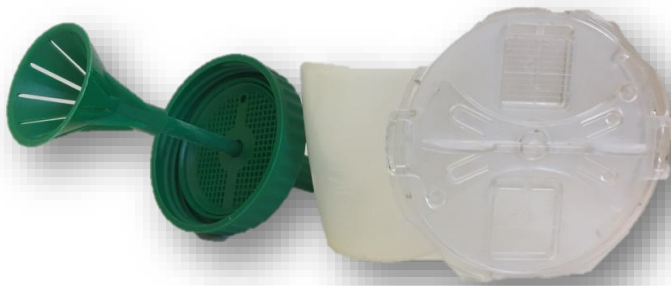
Figure 3 – Fill-FLOTAC with its sampling kit, filter and container and the reading disk, Mini-FLOTAC (Original)
