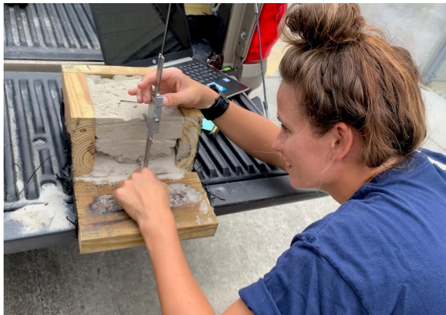
Figure 2-9. Depth test being conducted on sandbox sample.
