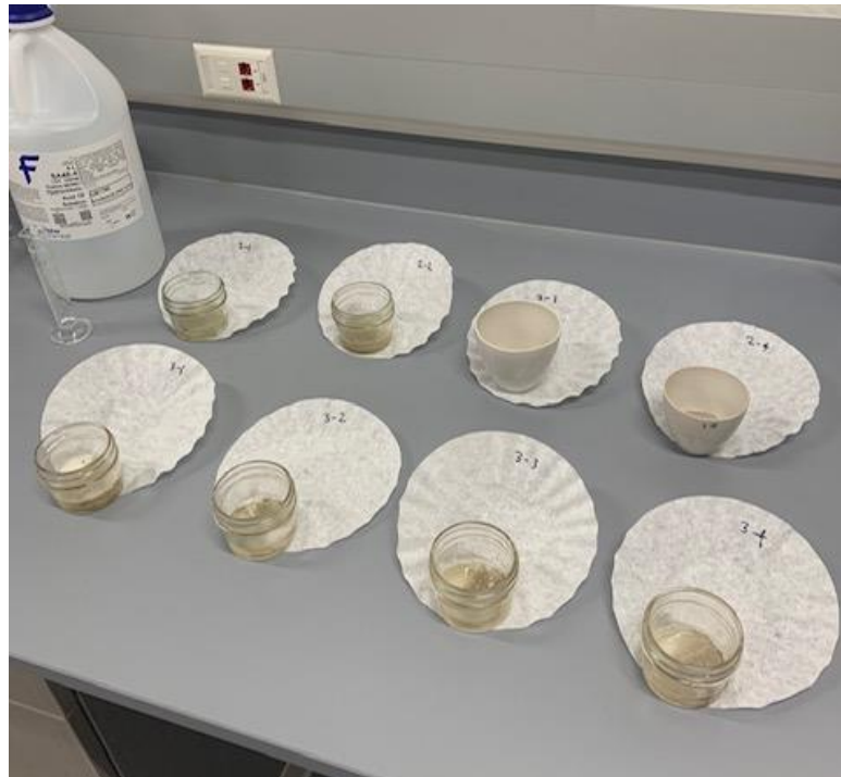
Figure 2-8. MICP treated soil mixing with HCl for a CCC test.
