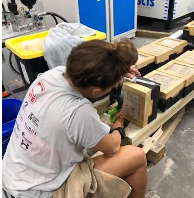
Figure 2-7. Pocket Erodrometer Test being conducted on MICP treated sandboxes
