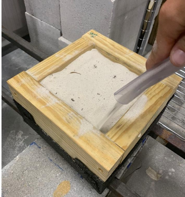
Figure 2-3. Air pluviating the sand for MICP treatment
