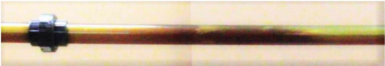
Figure 5.5: Slug Unit Length Measurement using High Speed Video Camera
