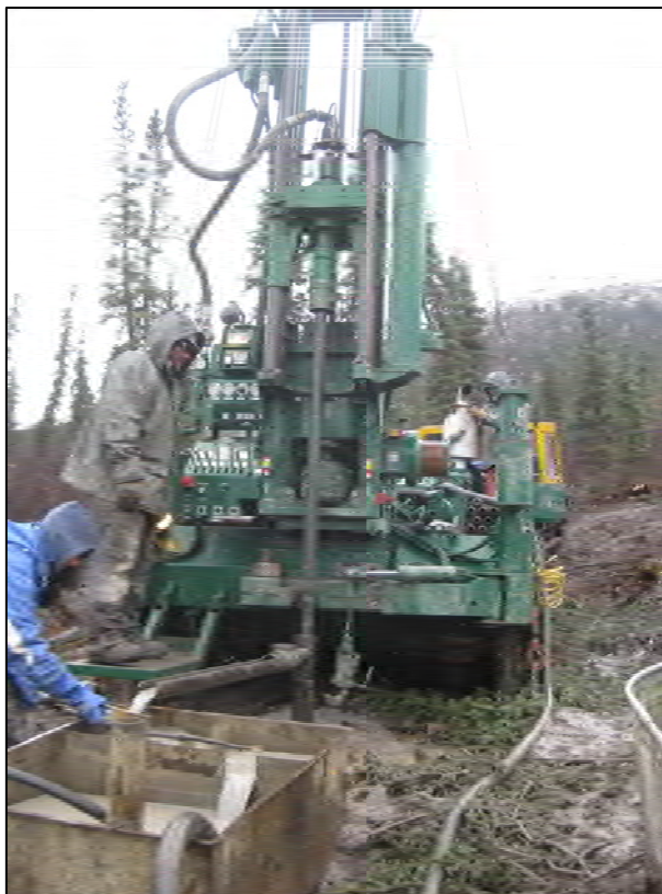
Figure B-2. Typical rig set-up for tricone and casing. Photograph taken while drilling TH12-9004. (Photograph by M. Darrow)
