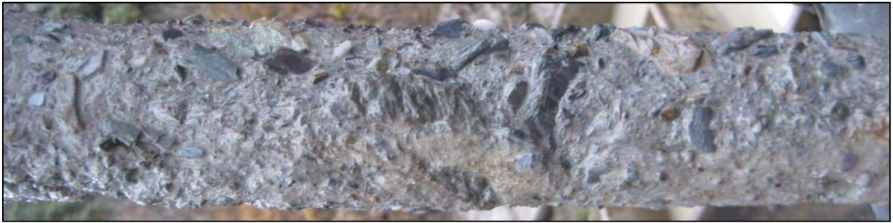
Figure 14. Example of frozen silty gravel typical of FDL-A. For scale, this photograph spans a 2-ft long split spoon sample. (Photograph by M. Darrow)
