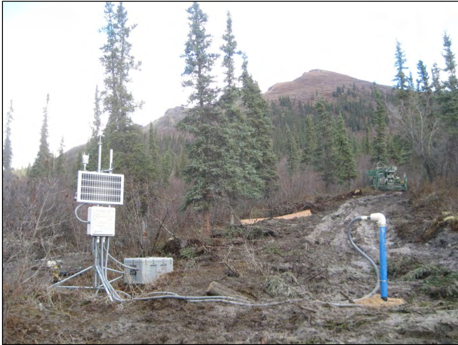
Figure B-9. Completed “main” ADAS location and casing installation of TH12-9004. (Photograph by M. Darrow)
