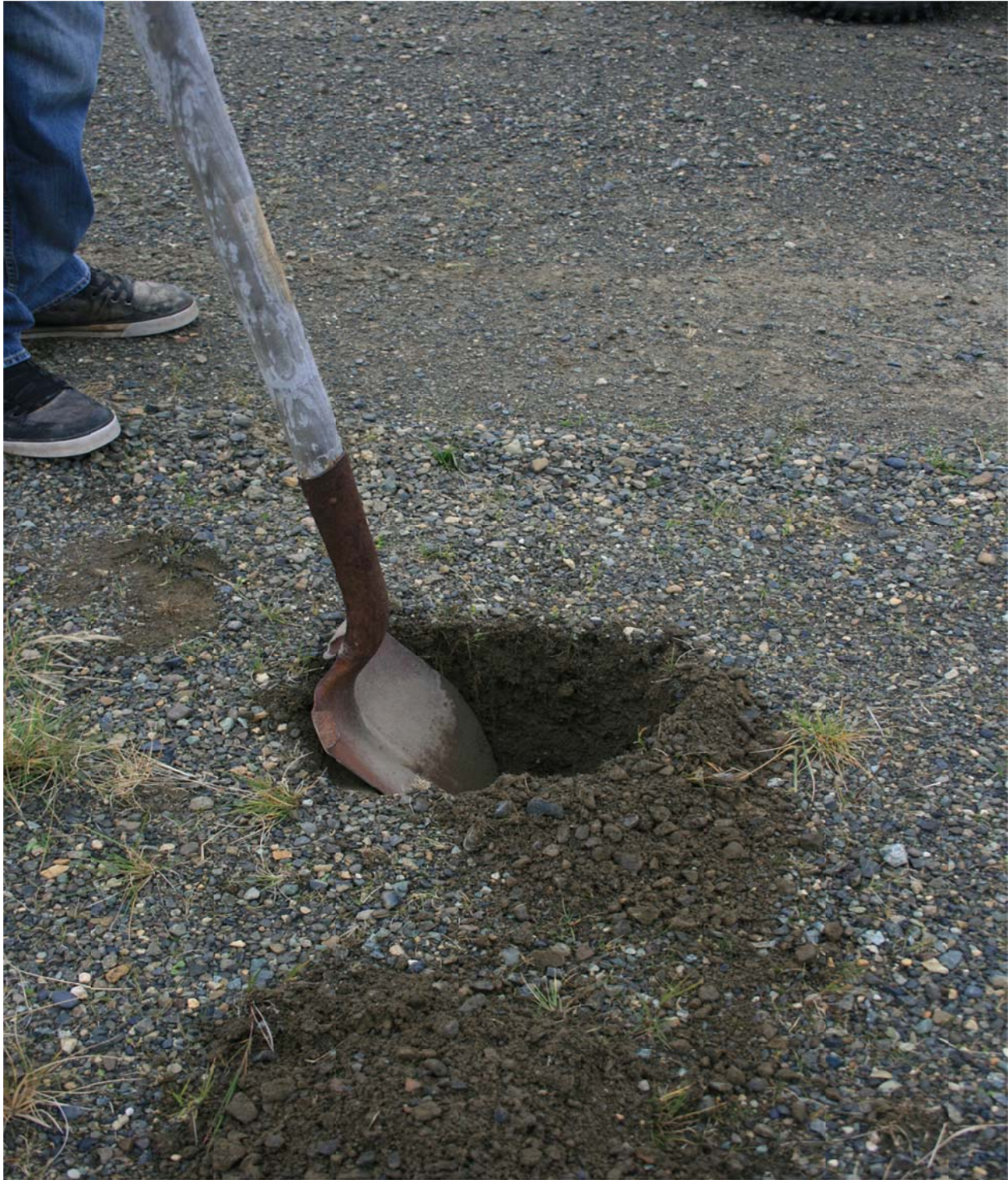
Figure 4: Hole on side of the runway showing a shallow depth of gravel
