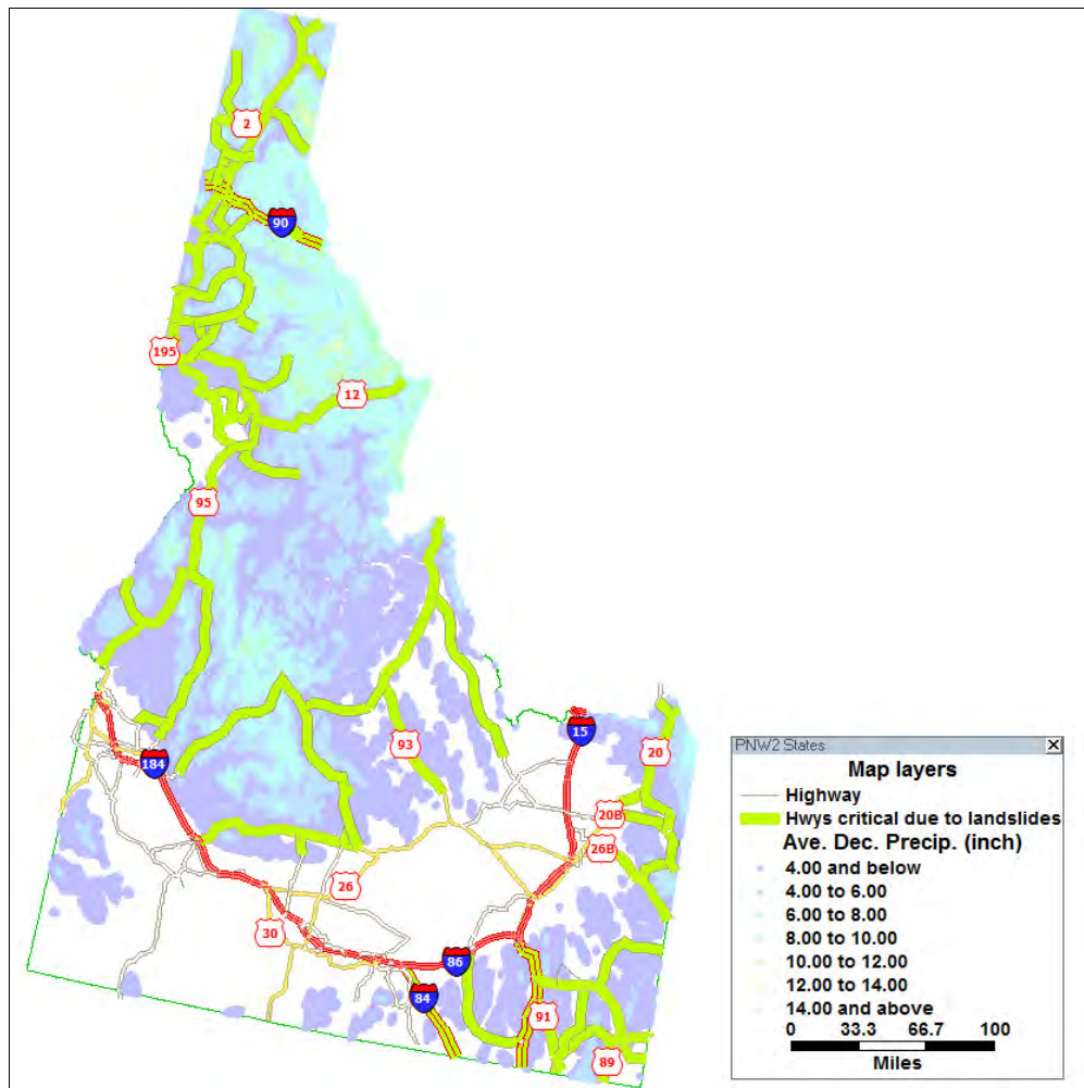
Figure 80 - Highways Located in Areas with Over 2 Inch Average December Precipitation in Idaho
