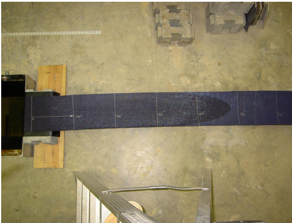
Figure 8. Water wicking of H2Ri at a zero hydraulic gradient
