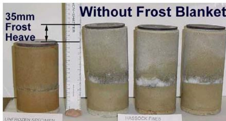
Figure 7. Components between soil specimens in the frost heave tests
