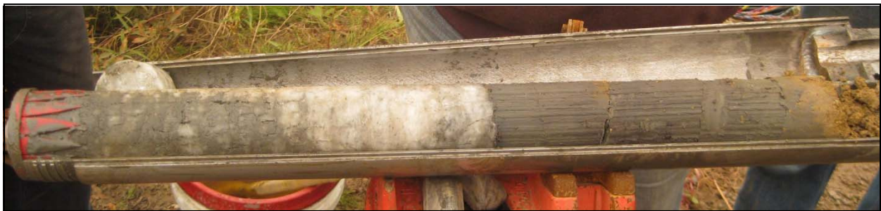
Figure 3.5. Split-spoon sample (11.0-13.0 ft bgs) from TH09-1402, showing transition from fill (at far right) to silt (right of center) to massive ice (left of center).
