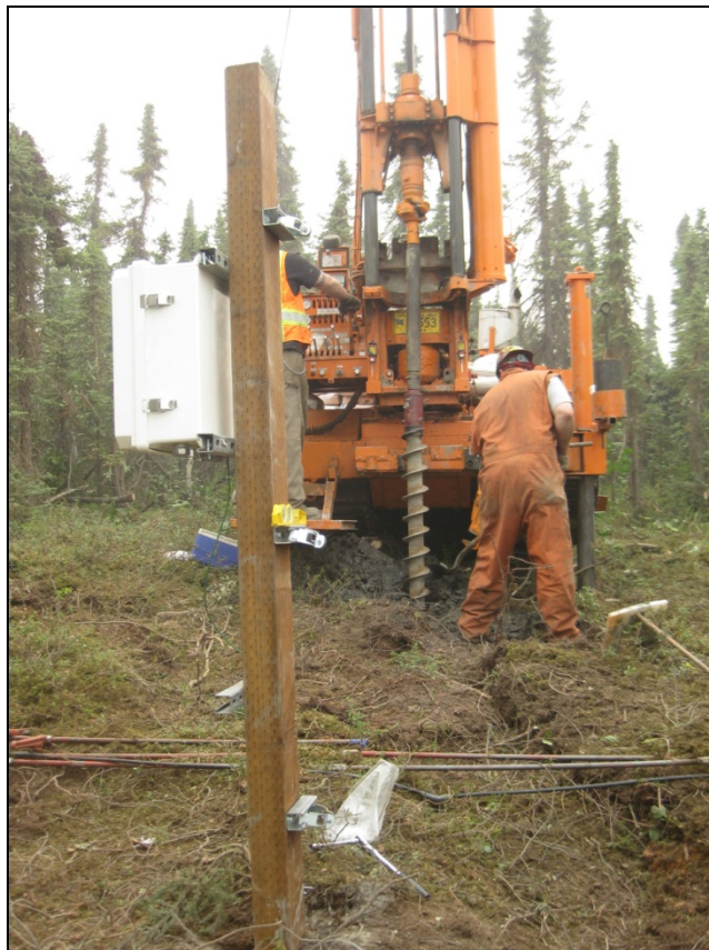
Figure 3.2. Drilling the boring for the undisturbed location, Dalton Highway 9 Mile Hill. Note the location of the post for the ADAS in the foreground.
