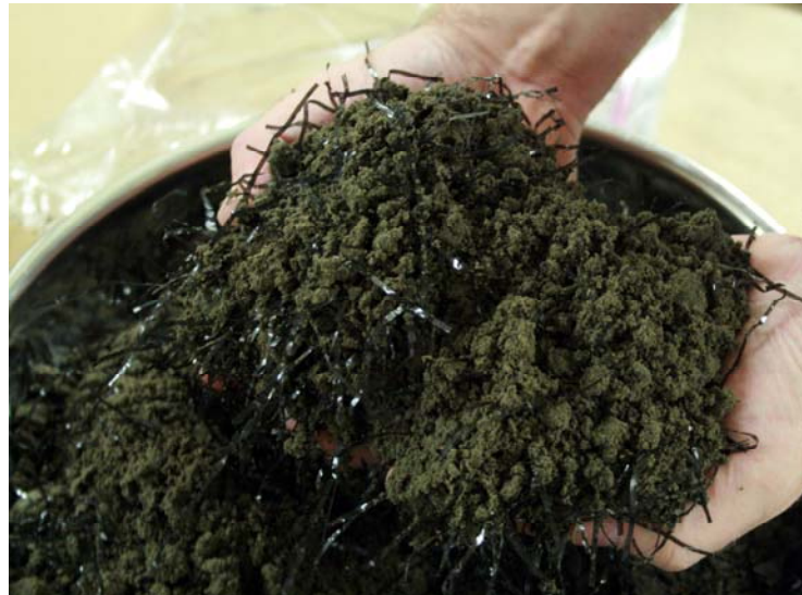
Figure 1: Sample mixture of soil, water, and geofibers.
