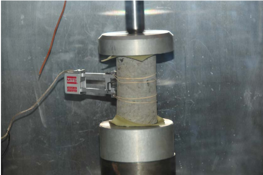
Figure 2.9 An extensometer attached to the middle of a frozen soil specimen during loading.
