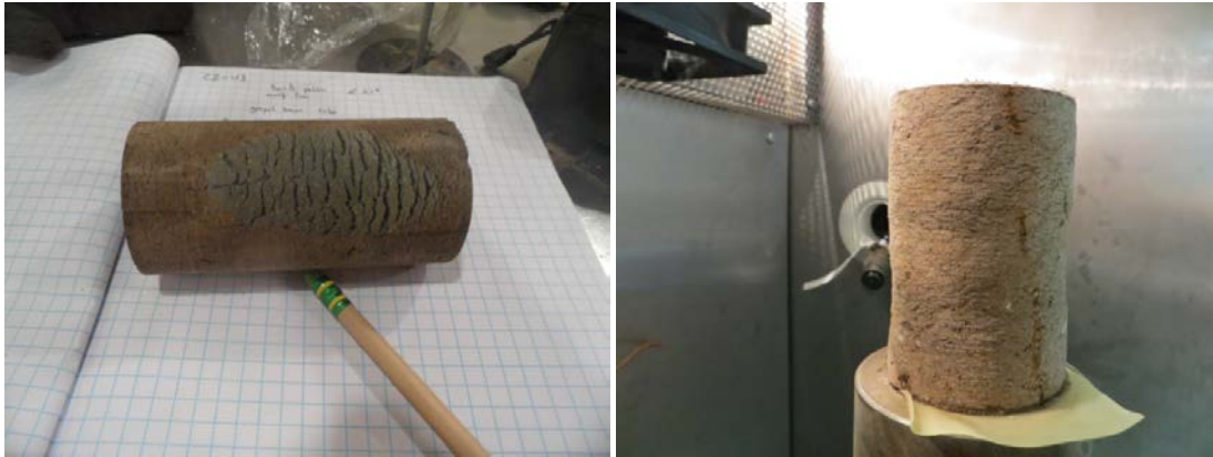
Figure 3.8 A vertically oriented naturally frozen soil cylinder with ice lenses: before testing (left) and after testing to 15% axial strain (right).
