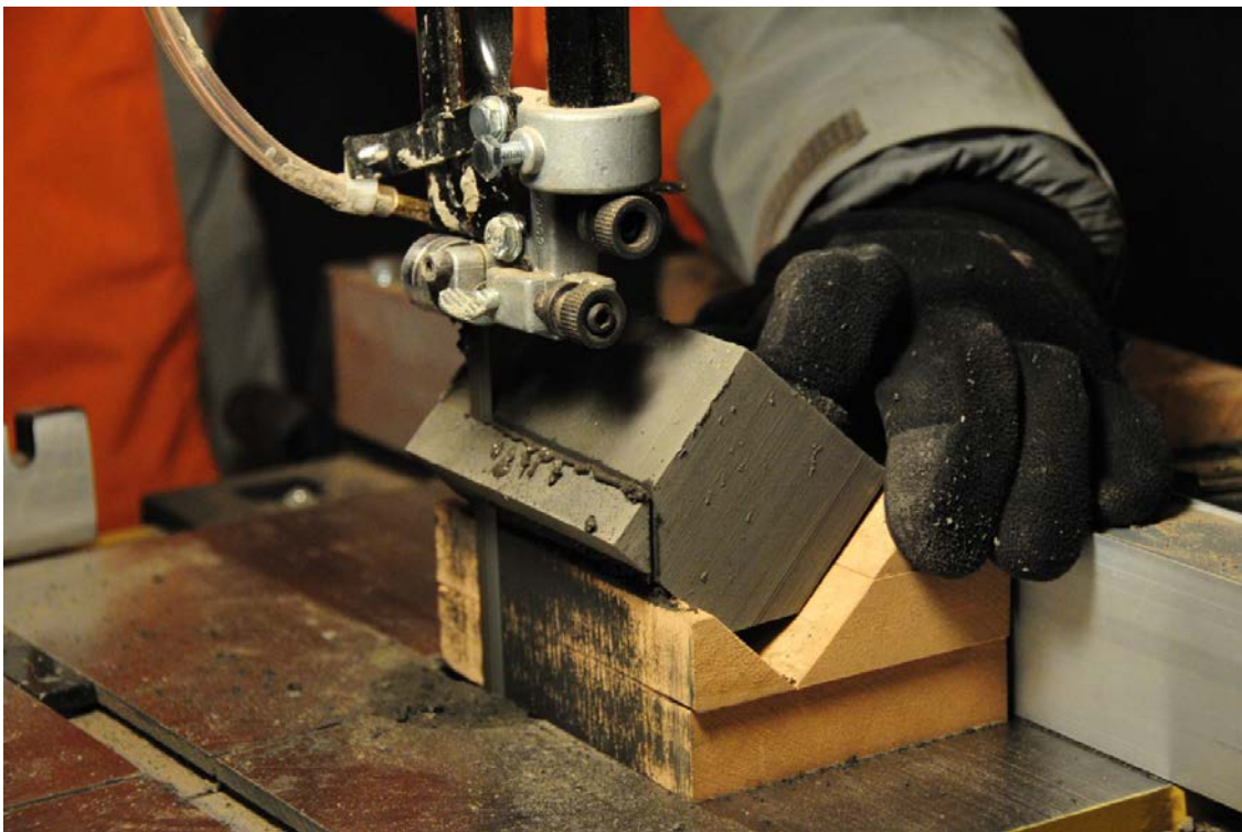
Figure 2.3 A frozen soil sample being cut into an octagon with the wood jig by a band saw.
