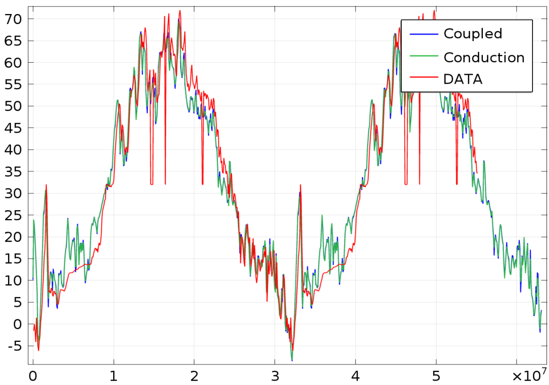
Figure 42. Modeled versus measured temperature data from a depth of 0.33 ft for the Part I 2D models. This data set was used to calibrate the side slope n -factors.
