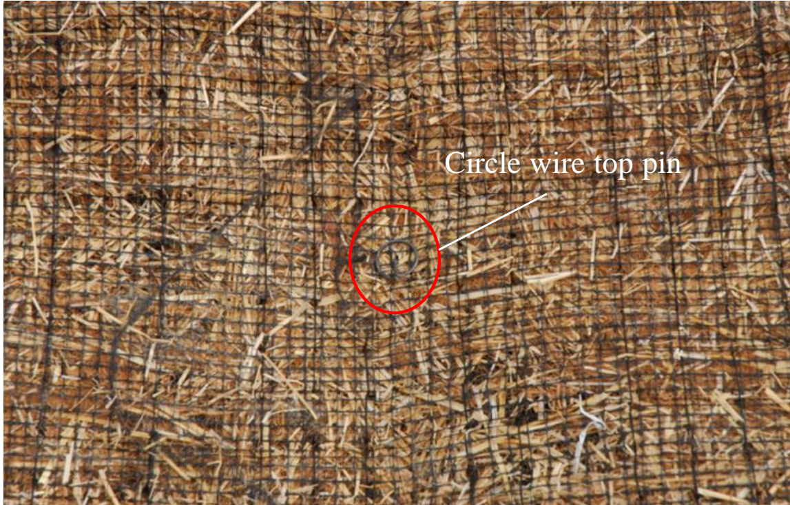
Figure 4.18 Enlargement of a circle wire top pin
