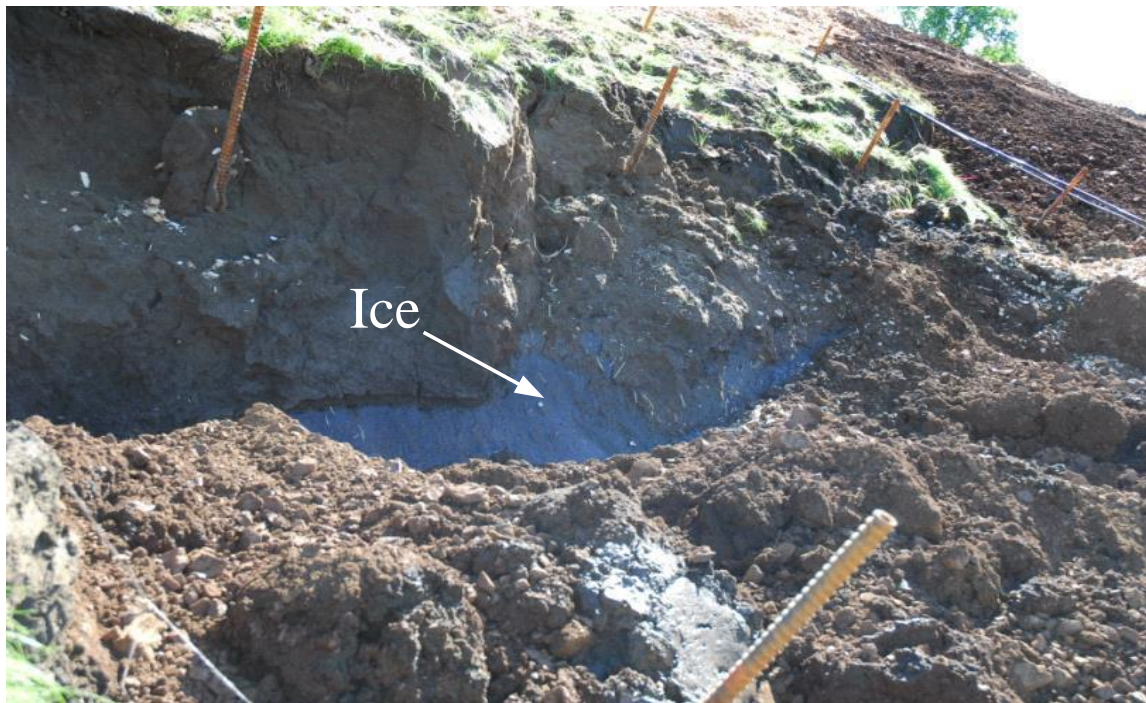
Figure 6.6 Massive ice in Section C
