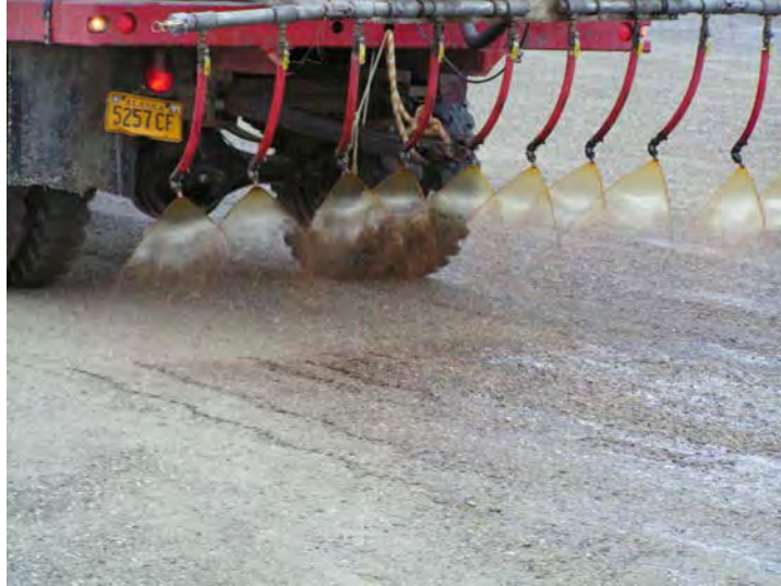
Figure 5.11 Uneven fan distribution
