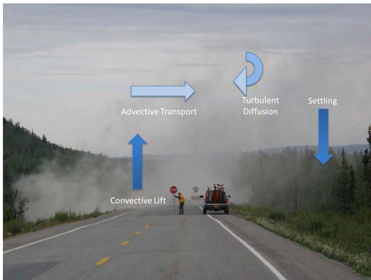
Figure 2.4. Process involved in particle movement and settling
