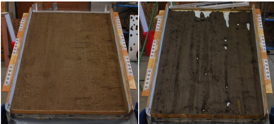
Fig. A-20: Before and After Pictures of 6% w + 2% SS – Test 2
