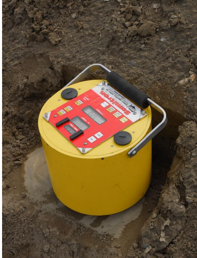
Fig. 3-15: GeoGauge testing at the field site
