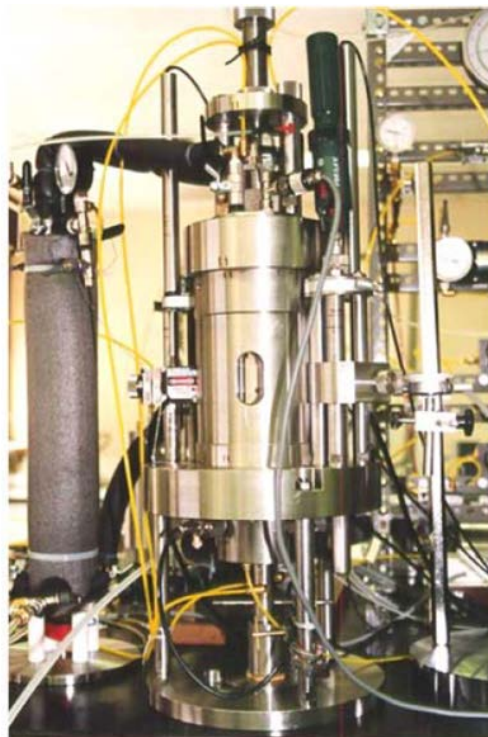
Figure 2.13 Laser scanner method setup (Romero et al. 1997)
