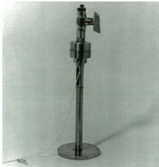
Figure 2.27 Tensiometer saturation device (Ridley and Burland 1993)
