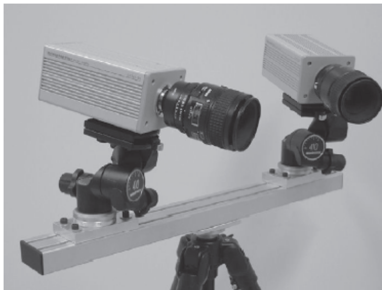
Figure 2.23 Configuration of the 3D DIC method (Orteu 2009)
