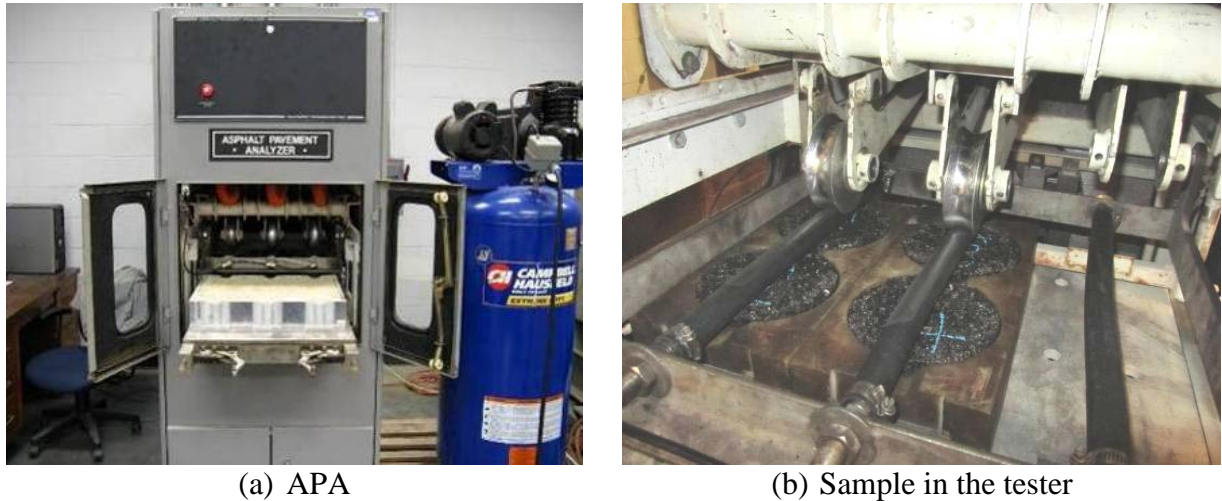
Figure 3.11 APA rutting susceptibility test
