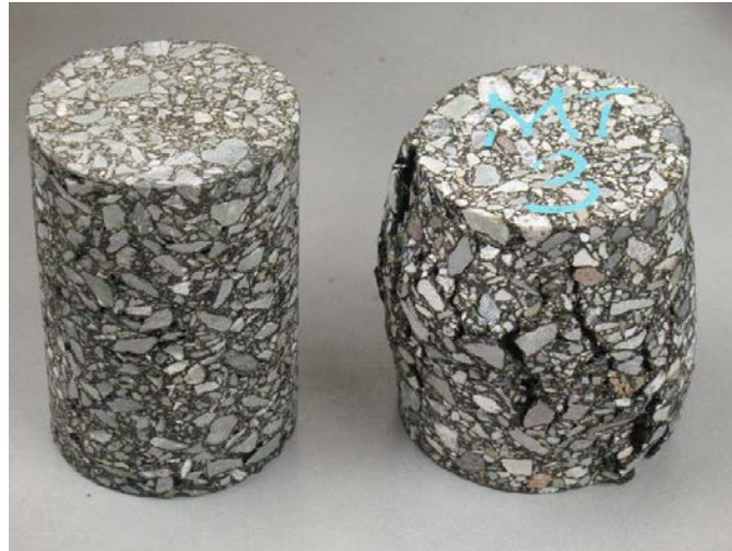
Figure 3.10 Specimens before and after the flow test
