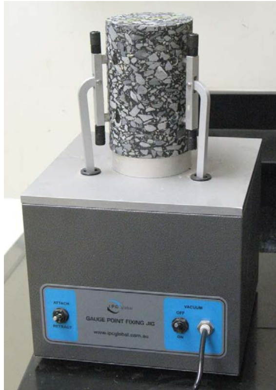
Figure 3.8 LVDT attachment apparatus
