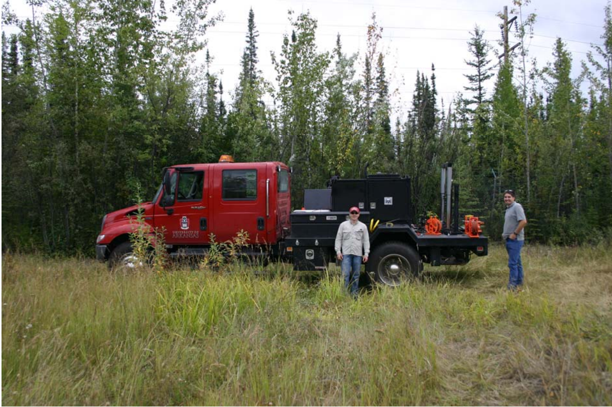
Figure 3 Photograph of The Hawg vibroseis truck owned and operated by the University of Arkansas.
