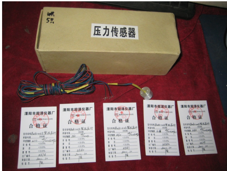
Figure 2.10. Pore pressure sensors
