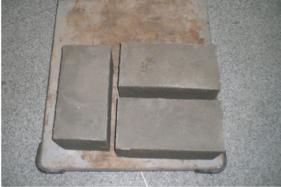
Figure 2.4. Cemented sand specimens
