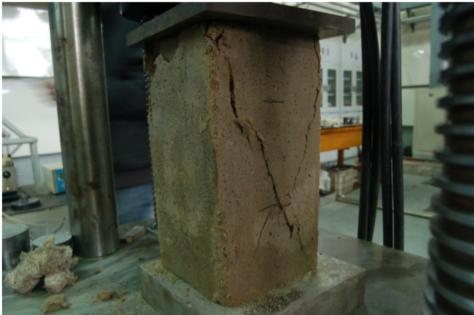
Figure 2.5. Snapshot of a uniaxial compression test of cemented sand specimen
