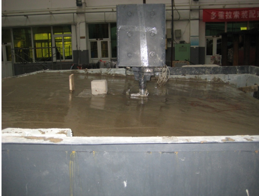
Figure 2.9. Cemented sands just placed for frozen crust simulation
