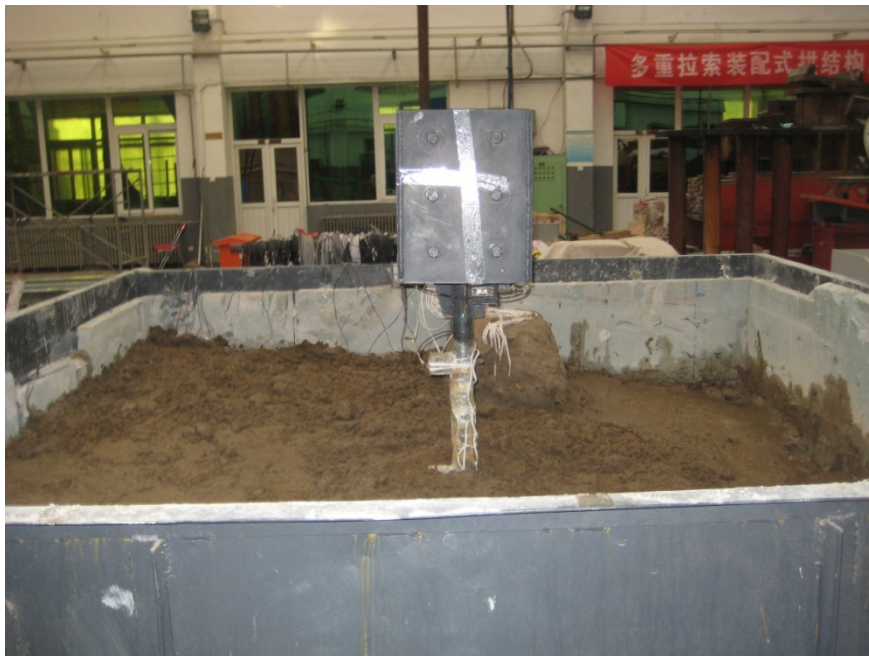
Figure 2.8. Smoothing the loose sand surface for placement of simulated frozen crust
