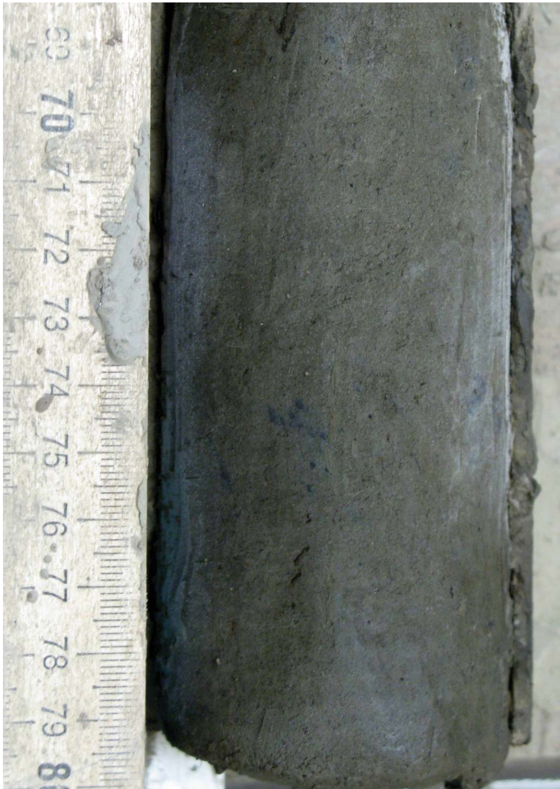
Figure 5.37. Silt with latent micro-lenticular cryostructure (inclined), borehole AUTC-5, depth 2.03-2.14 m, gravimetric moisture content 66%.
