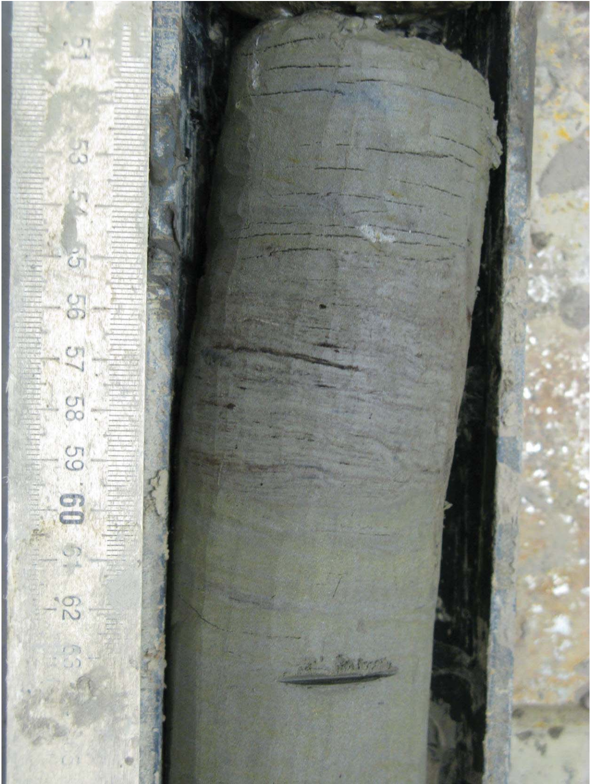
Figure 5.72. Ice-poor silt with layered – lenticular cryostructure, borehole AUTC-8, depth 14.28-14.43 m, gravimetric moisture content 36% (14.4-14.5 m, almost without visible ice).
