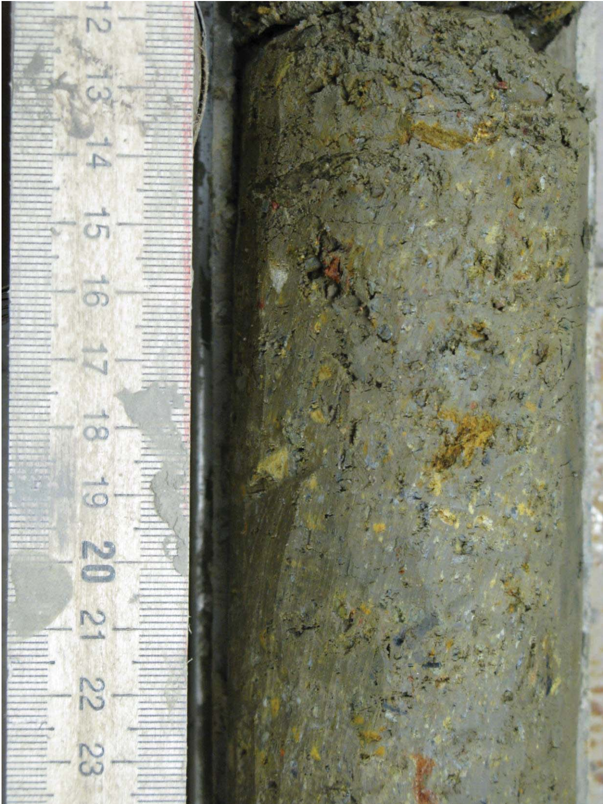
Figure 5.52. Gravelly sandy silt (epigenetic permafrost) with crustal cryostructure, borehole AUTC-6, depth 18.67-18.77 m, gravimetric moisture content 24%.
