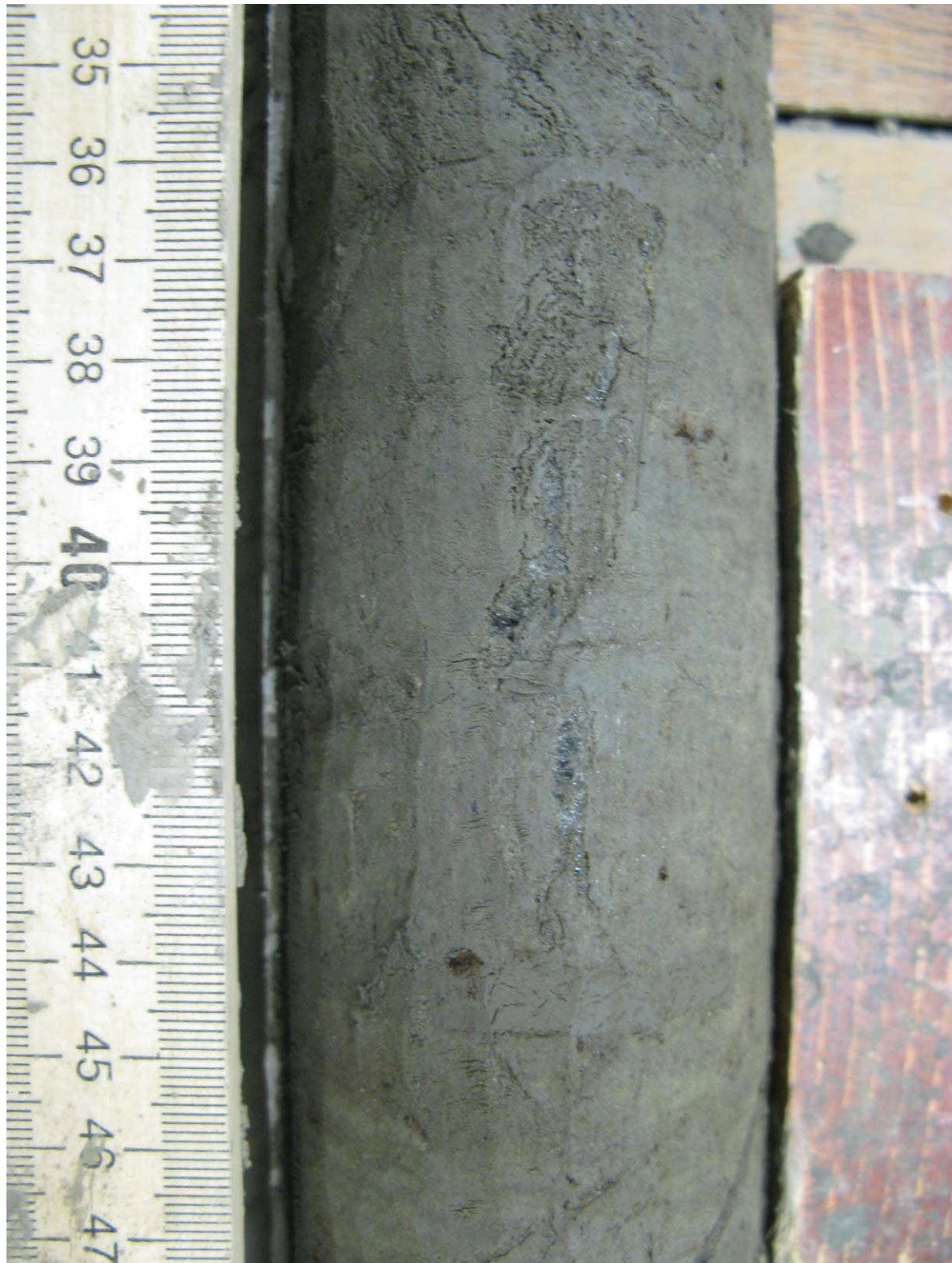
Figure 5.13. Silt with small ice vein, typical of syngenetic permafrost, borehole AUTC-2, depth 11.43-11.55 m.
