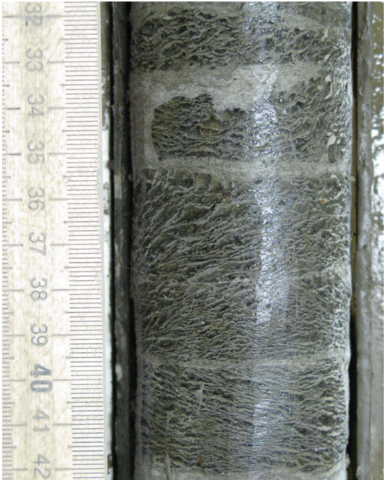
Figure 5.19. Silt with micro-ataxitic – micro-braided cryostructure, borehole AUTC-3, depth 5.62-5.72 m, gravimetric moisture content 233%.
