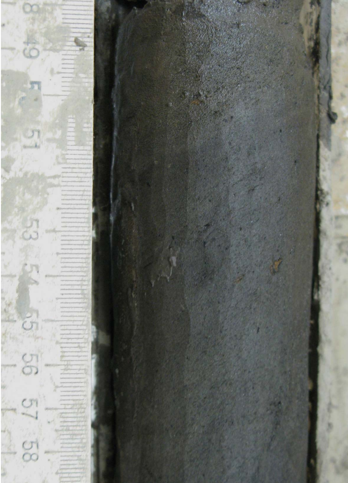
Figure 5.71. Silt with micro-braided – micro-lenticular cryostructure, inclined, borehole AUTC-8, depth 6.9-7.0 m, gravimetric moisture content 118%.
