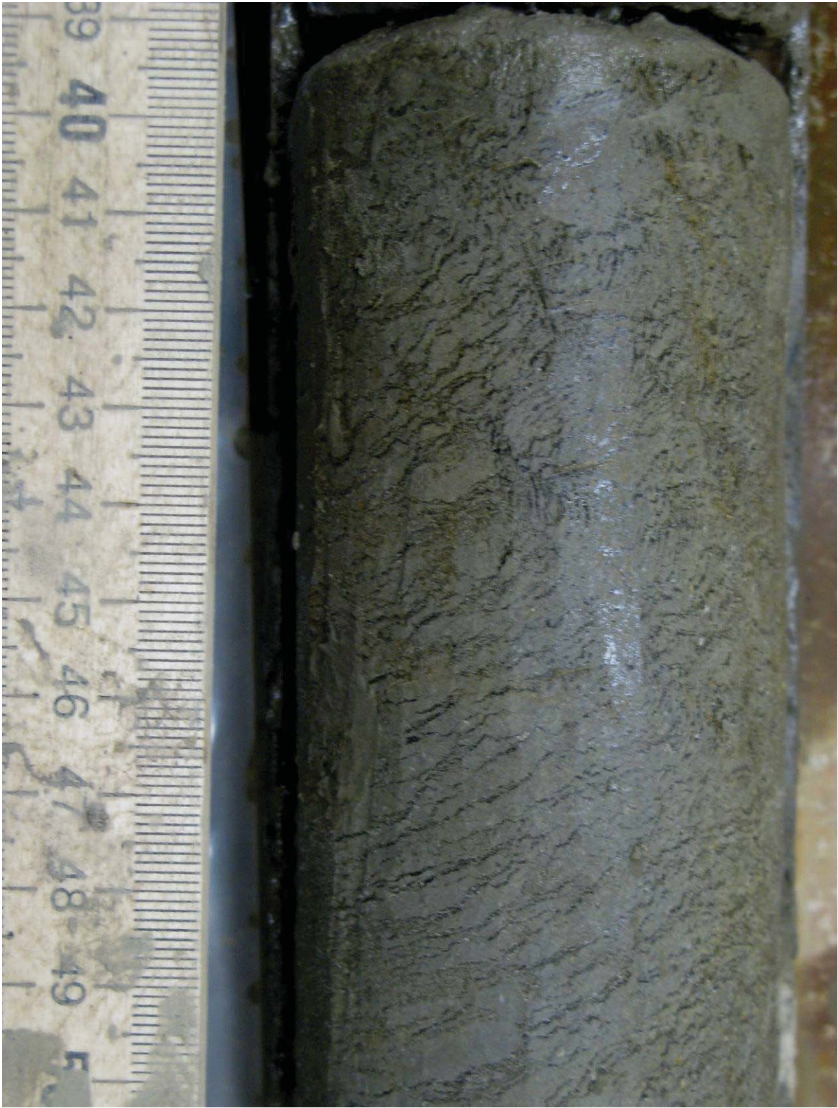
Figure 5.61. Silt with braided – micro-braided cryostructure, borehole AUTC-7, depth 11.5-11.6 m, gravimetric moisture content 73%.
