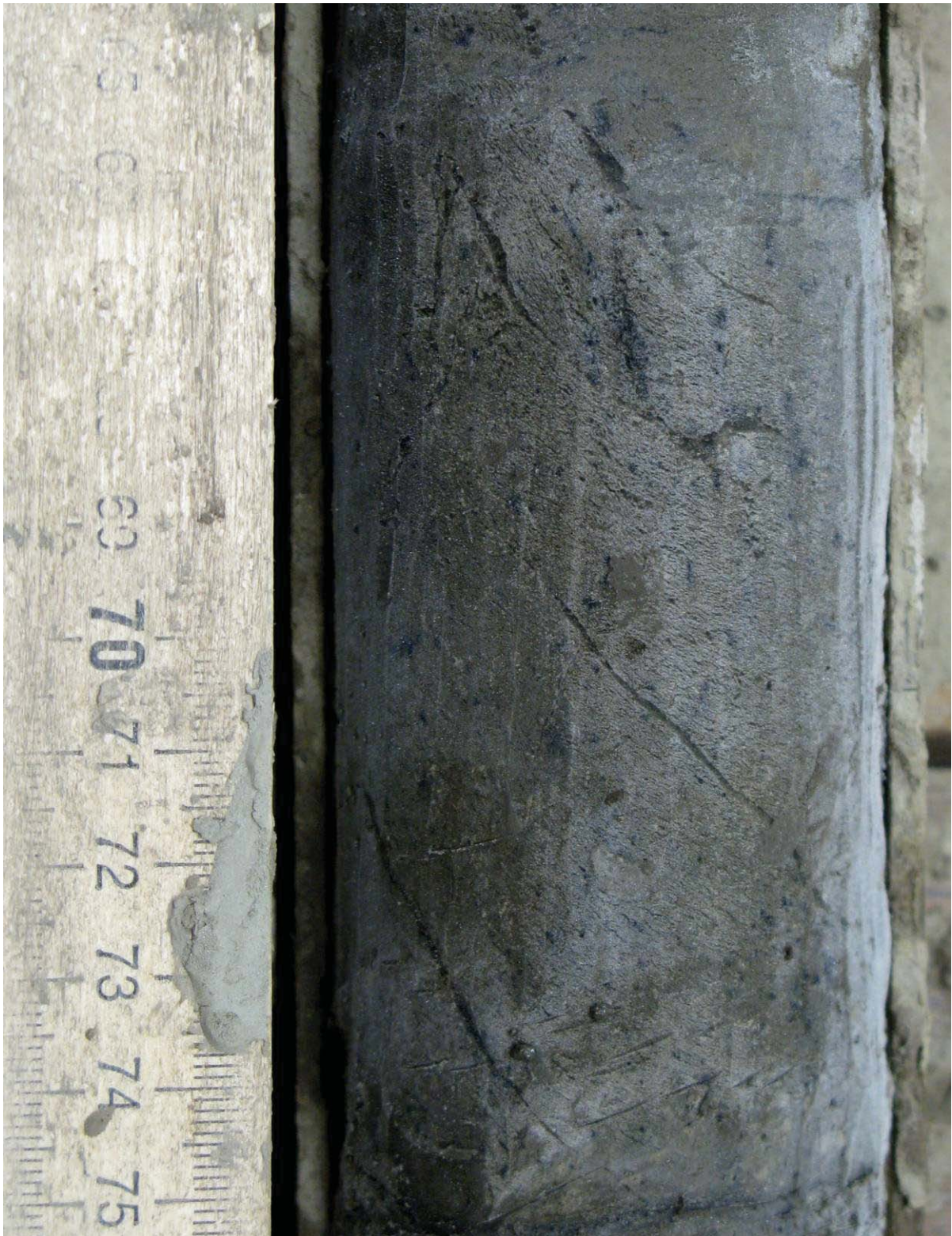
Figure 5.29. Silt with micro-lenticular – micro-braided cryostructure, borehole AUTC-4, depth 8.15-8.25 m, gravimetric moisture content 92%. Note inclination of ice lenses indicating proximity of ice wedge.
