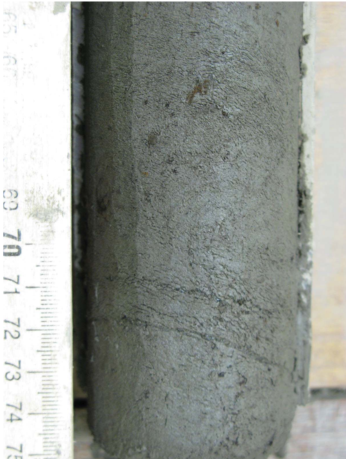
Figure 5.12. Silt with micro-lenticular – micro-braided cryostructure, borehole AUTC-2, depth 10.95-11.05 m, gravimetric moisture content 81%.
