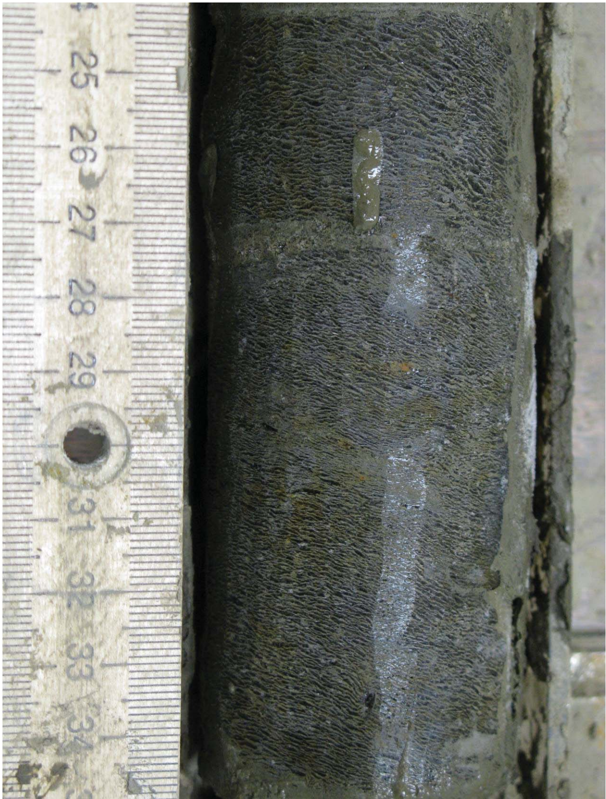
Figure 5.27. Silt with micro-braided – micro-ataxitic cryostructure, borehole AUTC-4, depth 0.84-0.95 m.
