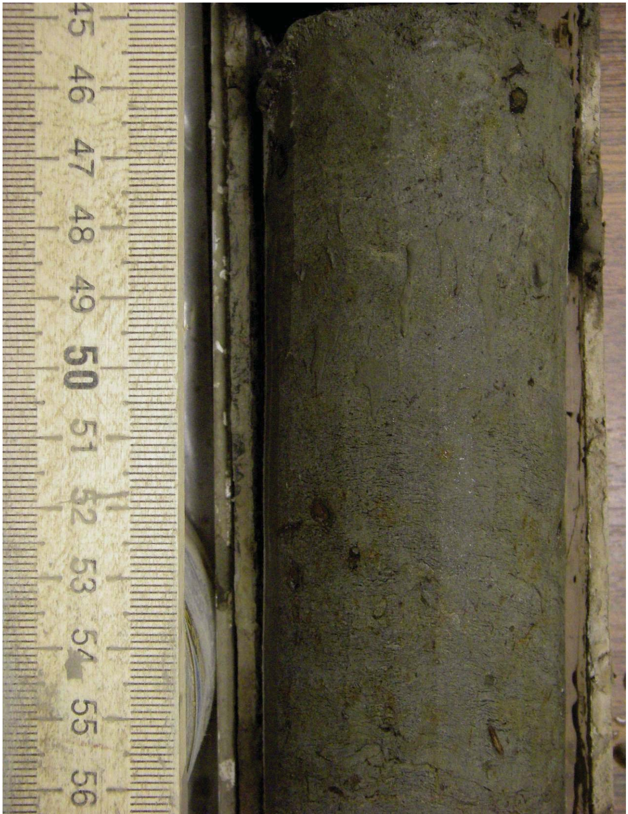
Figure 5.80. Silt with latent micro-lenticular – micro-lenticular cryostructure, borehole AUTC-9, depth 17.44-17.55 m, gravimetric moisture content 51%.
