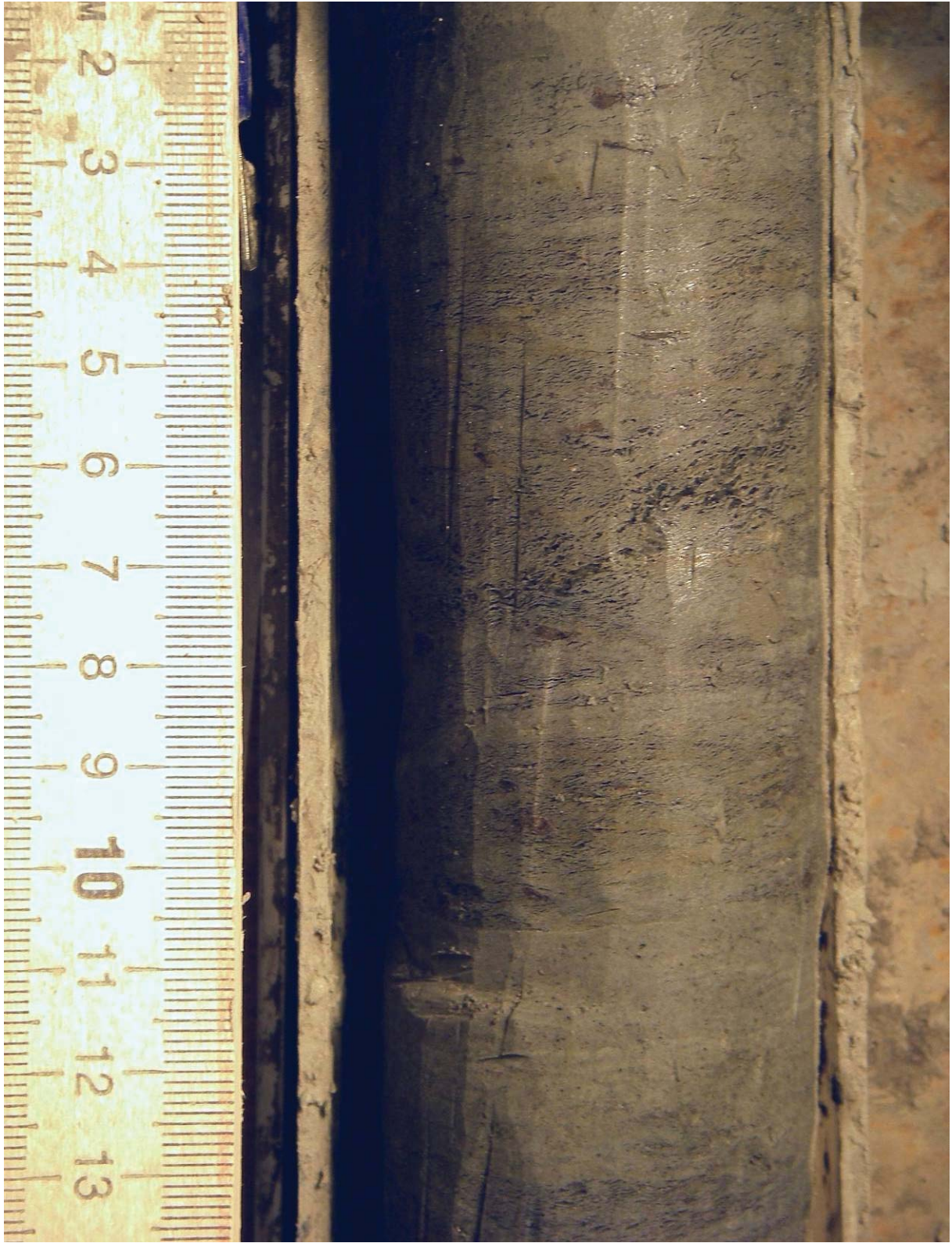
Figure 5.81. Silt with micro-braided – micro-lenticular cryostructure, borehole AUTC-9, depth 19.16-19.28 m, gravimetric moisture content 81%.
