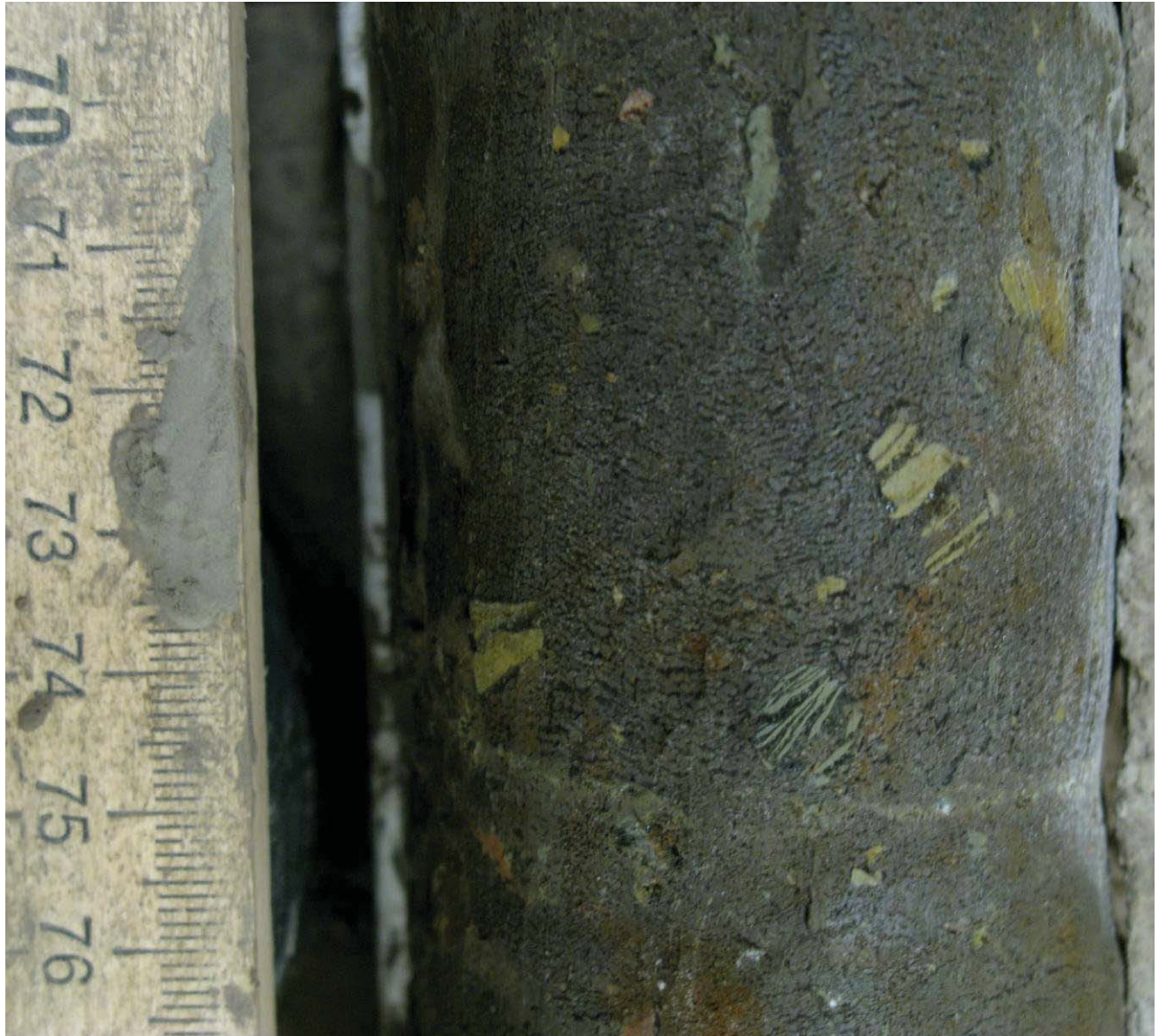
Figure 5.30. Silt with coarse sand and gravel, with crustal / micro-braided cryostructure, borehole AUTC-4, depth 9.63-9.70 m, gravimetric moisture content 67%.
