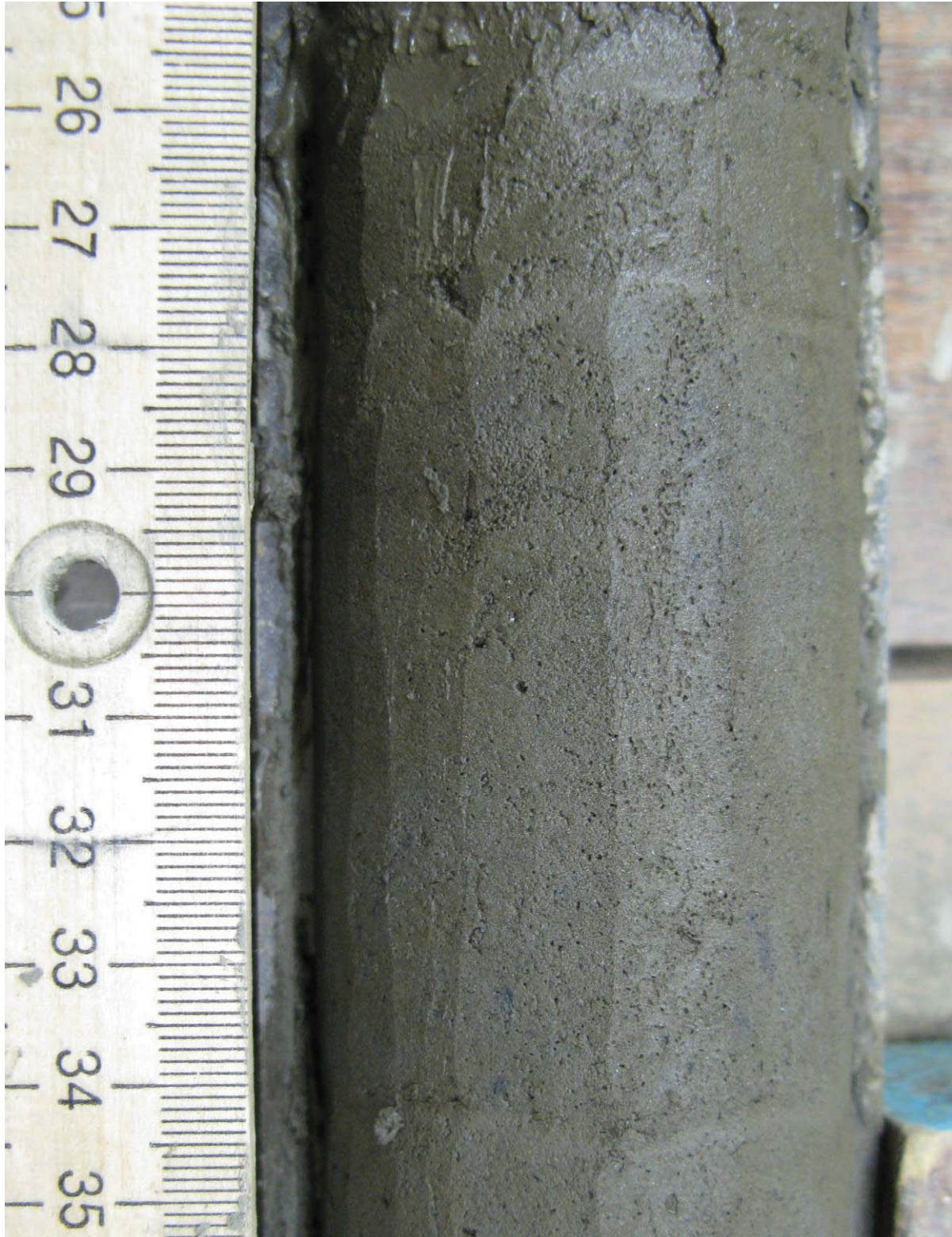
Figure 5.11. Silt with micro-porphyrific cryostructure, borehole AUTC-2, depth 9.2-9.3 m, gravimetric moisture content 64%.
