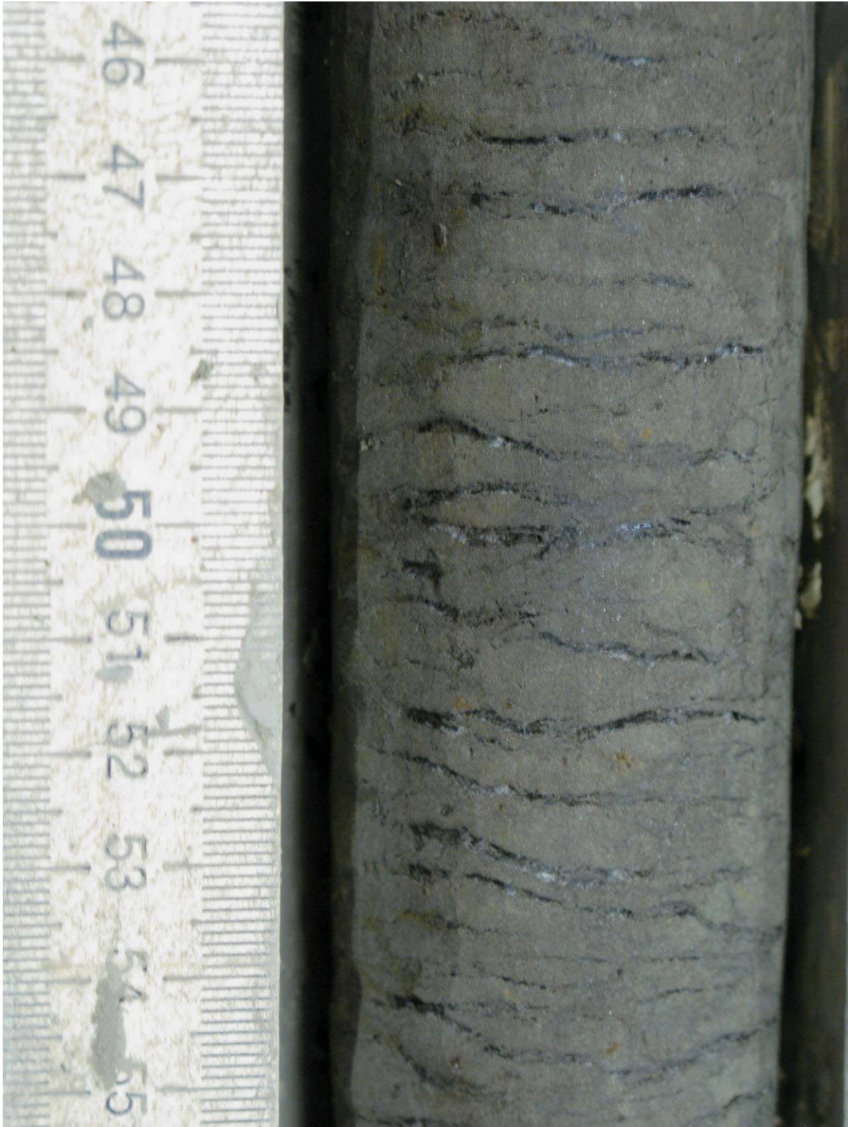
Figure 5.21. Silt with layered – braided cryostructure, borehole AUTC-3, depth 6.65-6.75 m, gravimetric moisture content 45%.
