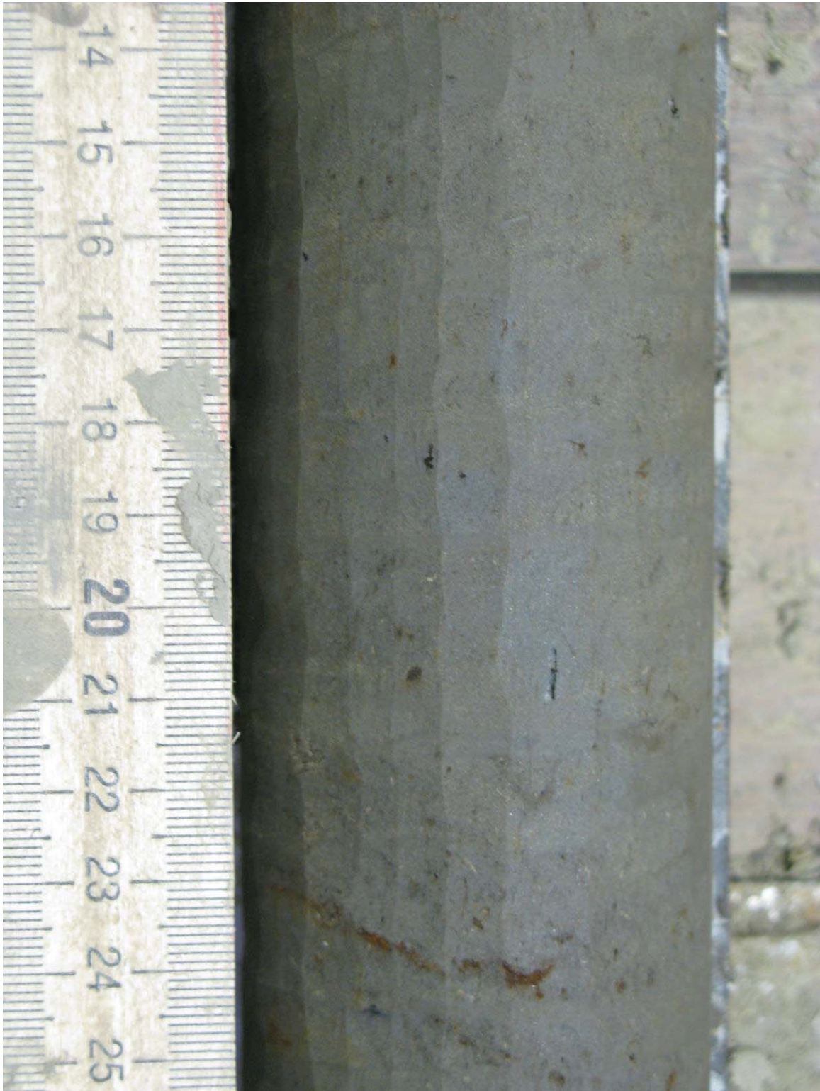
Figure 5.47. Silt with porous cryostructure (no visible ice), borehole AUTC-6, depth 2.25-2.36 m, gravimetric moisture content 39%.
