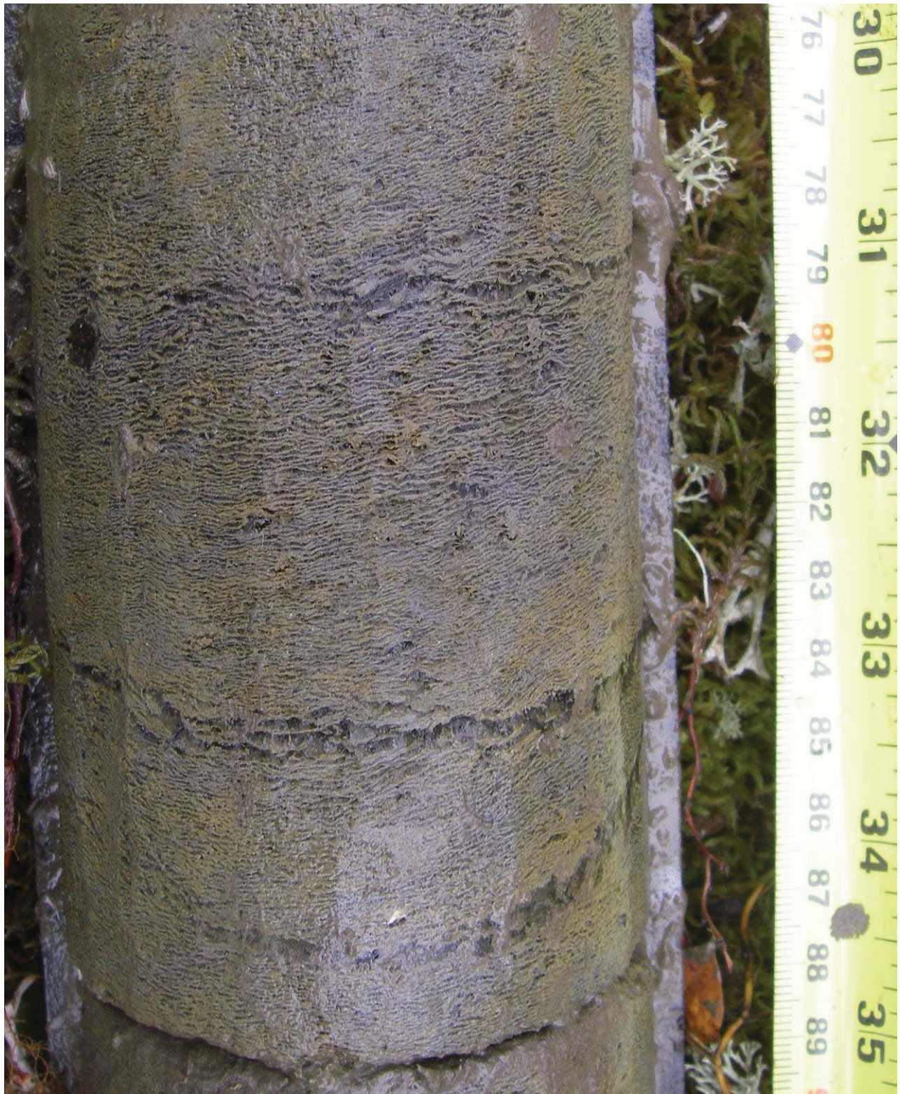
Figure 3.8. Belt-like cryostructure (combined with micro-braided cryostructure) of syngenetic permafrost (Dalton Highway innovation project area, Interior Alaska).
