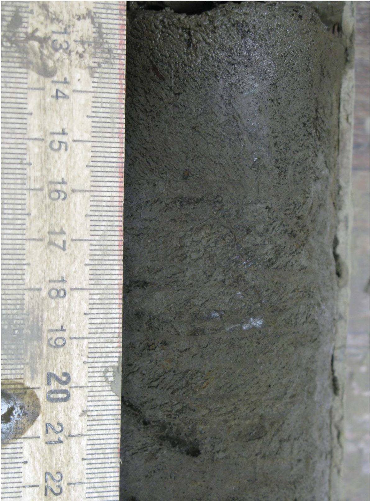
Figure 5.39. Silt with micro-lenticular – micro-braided cryostructure, borehole AUTC-5, depth 4.55-4.64 m, gravimetric moisture content 90%.
