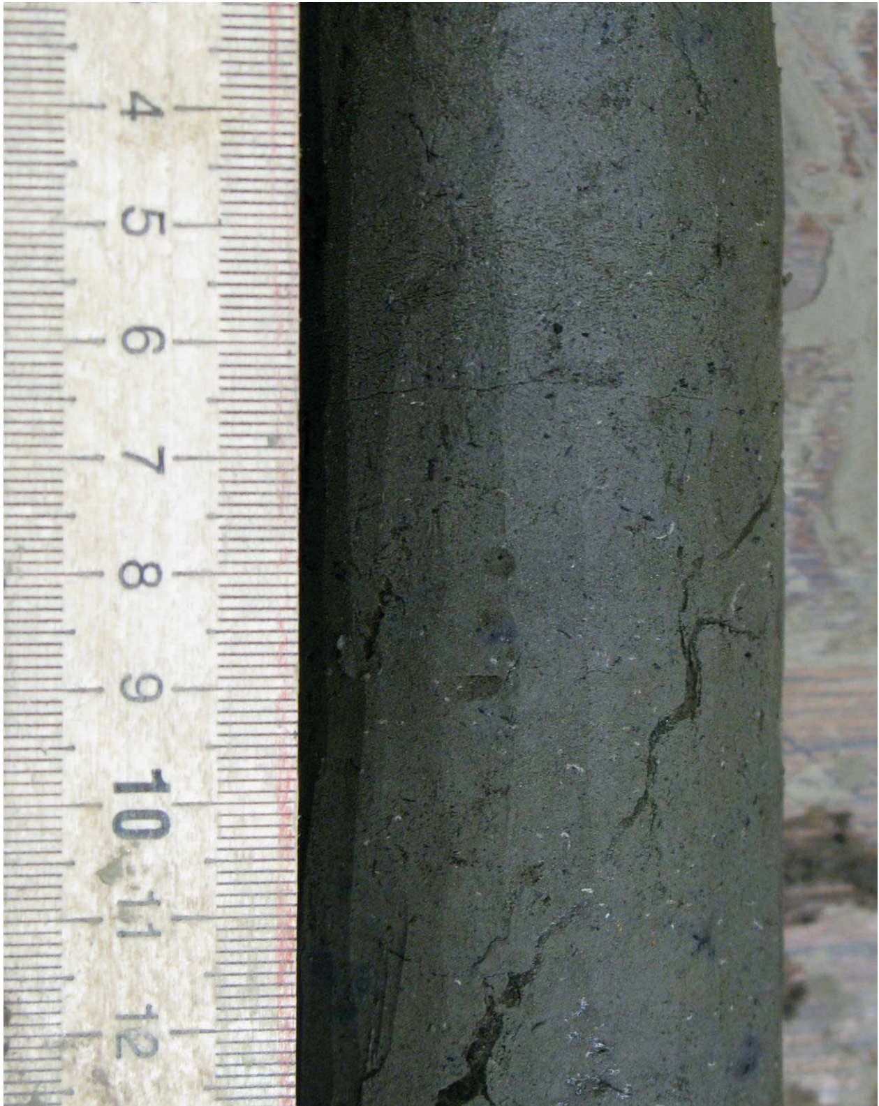
Figure 5.79. Silt with latent micro-lenticular – micro-porphyrific cryostructure, with small ice veins, borehole AUTC-9, depth 13.75-13.85 m, gravimetric moisture content 62%.
