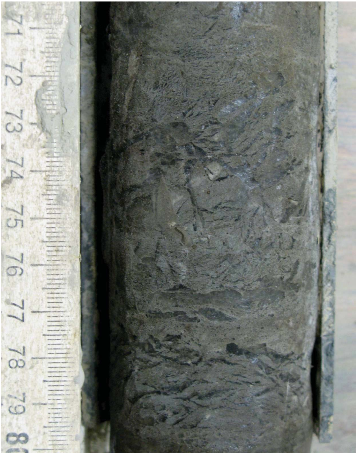
Figure 5.58. Silt with reticulate – braided cryostructure, borehole AUTC-7, depth 2.66-2.76 m, gravimetric moisture content 157%.
