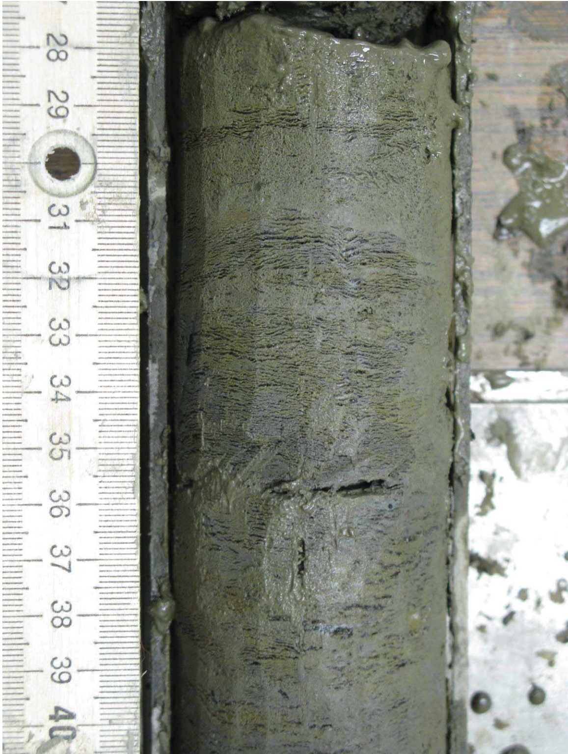
Figure 5.17. Silt with micro-braided – micro-lenticular cryostructure, borehole AUTC-3, depth 1.03-1.15 m.
