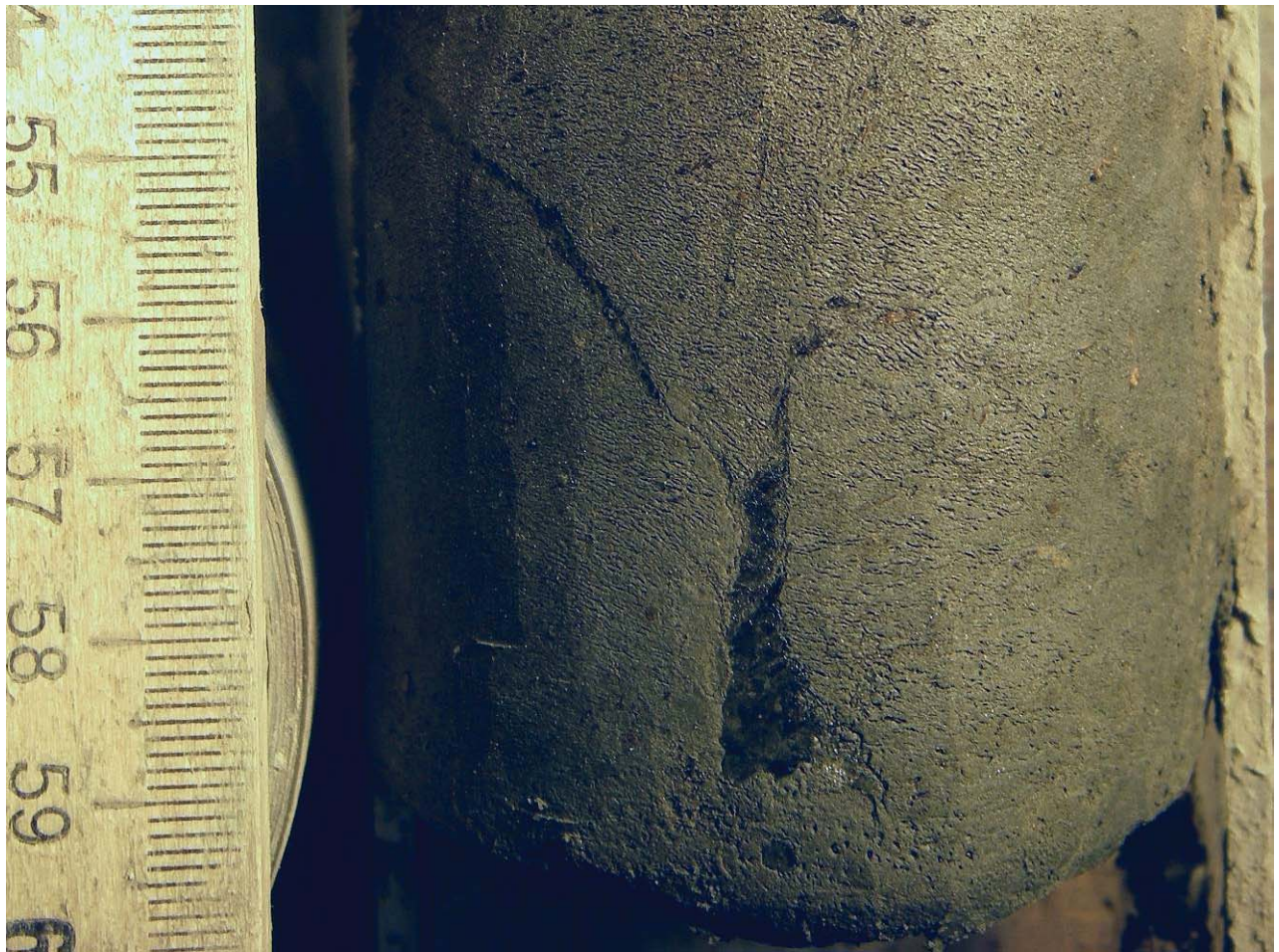
Figure 5.82. Silt with micro-braided – micro-lenticular cryostructure, with ice veins, borehole AUTC-9, depth 21.30-21.35 m, gravimetric moisture content 90%.
