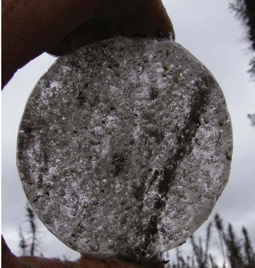
Figure 3.2. Appearance of wedge-ice, sample obtained by coring (Dalton Highway innovation project area, Interior Alaska).
