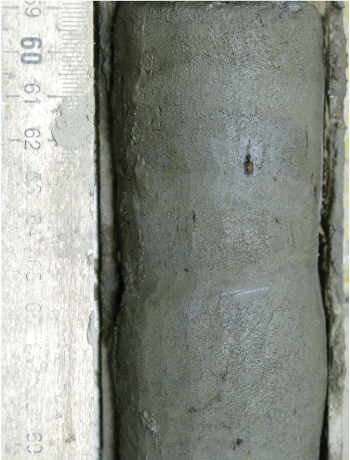
Figure 5.38. Silt with latent micro-lenticular cryostructure, borehole AUTC-5, depth 2.74-2.85 m, gravimetric moisture content 74%.
