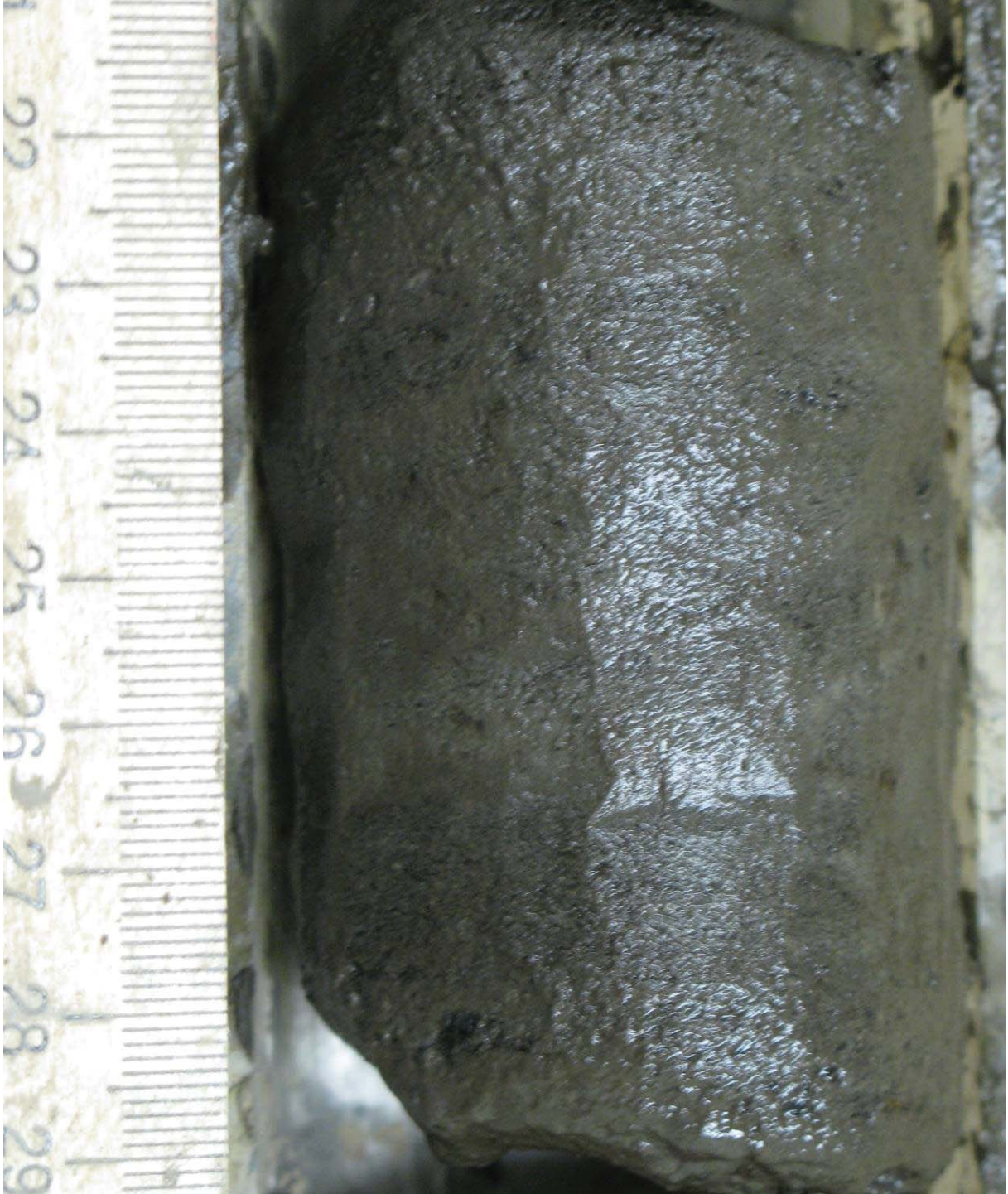
Figure 5.59. Organic silt with micro-braided cryostructure, borehole AUTC-7, depth 3.00-3.08 m, gravimetric moisture content 183%.
