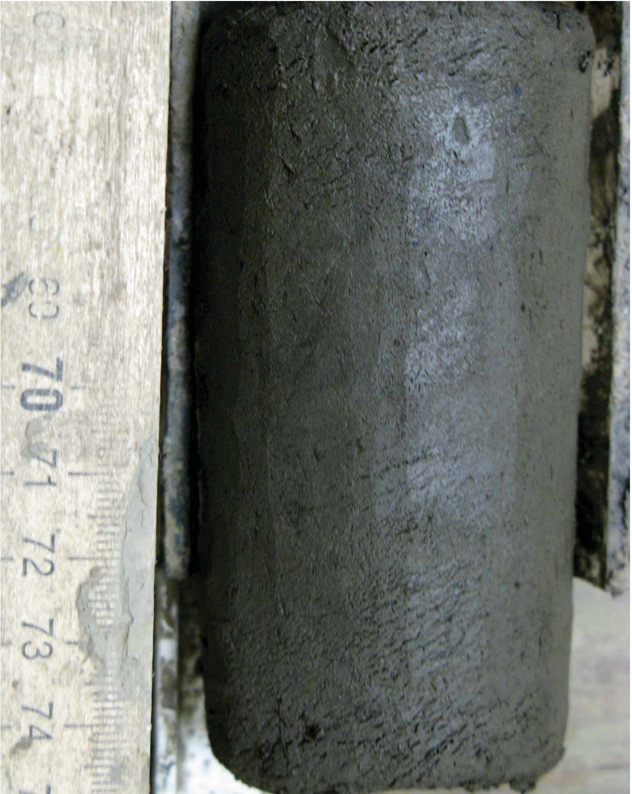
Figure 5.60. Silt with micro-lenticular – micro-braided cryostructure, borehole AUTC-7, depth 4.25-4.35 m, gravimetric moisture content 81%.
