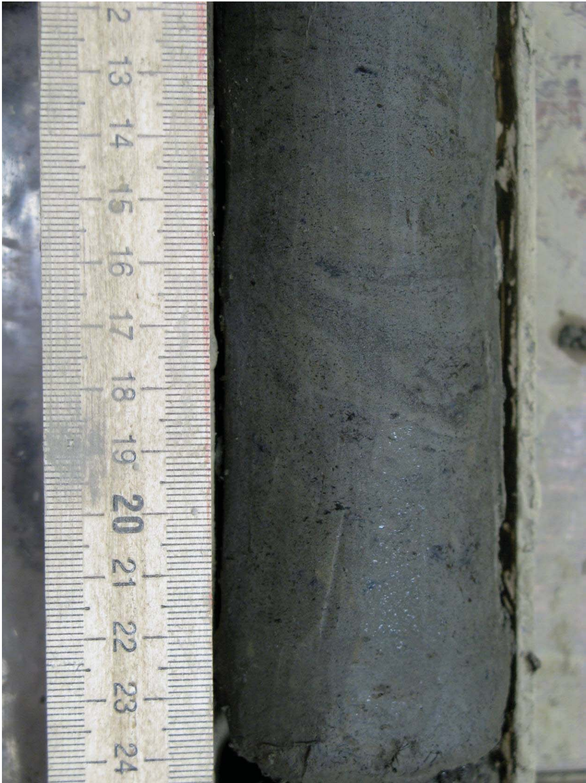
Figure 5.28. Silt with micro-porphyrific cryostructure, borehole AUTC-4, depth 3.16-3.28 m, gravimetric moisture content 47%.
