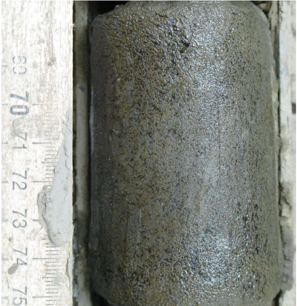
Figure 5.40. Silt with micro-ataxitic – micro-braided cryostructure, borehole AUTC-5, depth 7.30-7.38 m, gravimetric moisture content 126%.
