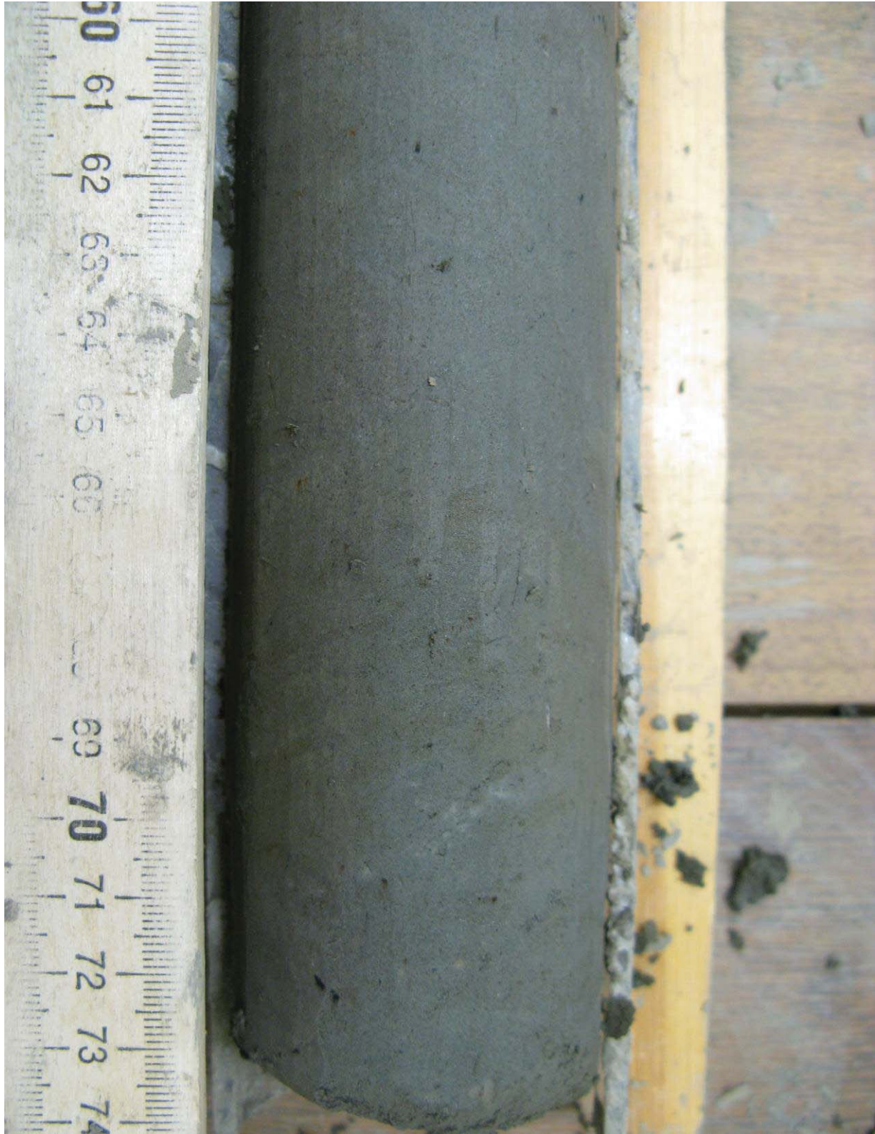
Figure 5.9. Silt with porous cryostructure (no visible ice), borehole AUTC-2, depth 7.20-7.44 m, gravimetric moisture content 45%.
