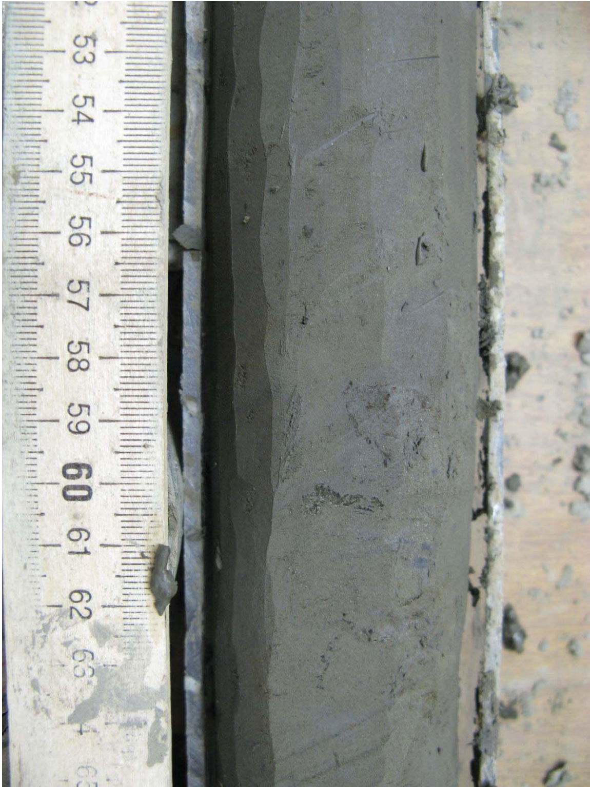
Figure 5.10. Silt with porous cryostructure (no visible ice), borehole AUTC-2, depth 8.60-8.73 m, gravimetric moisture content 45%.
