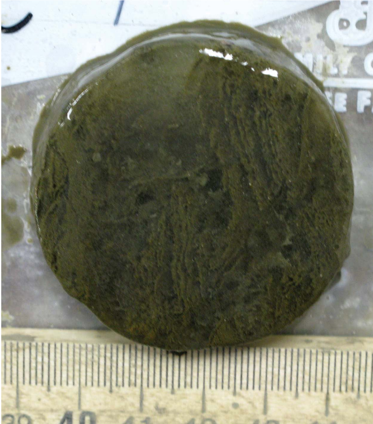
Figure 5.63. Sediment-rich wedge-ice with vertical foliation, borehole AUTC-7, depth 11.9 m.
