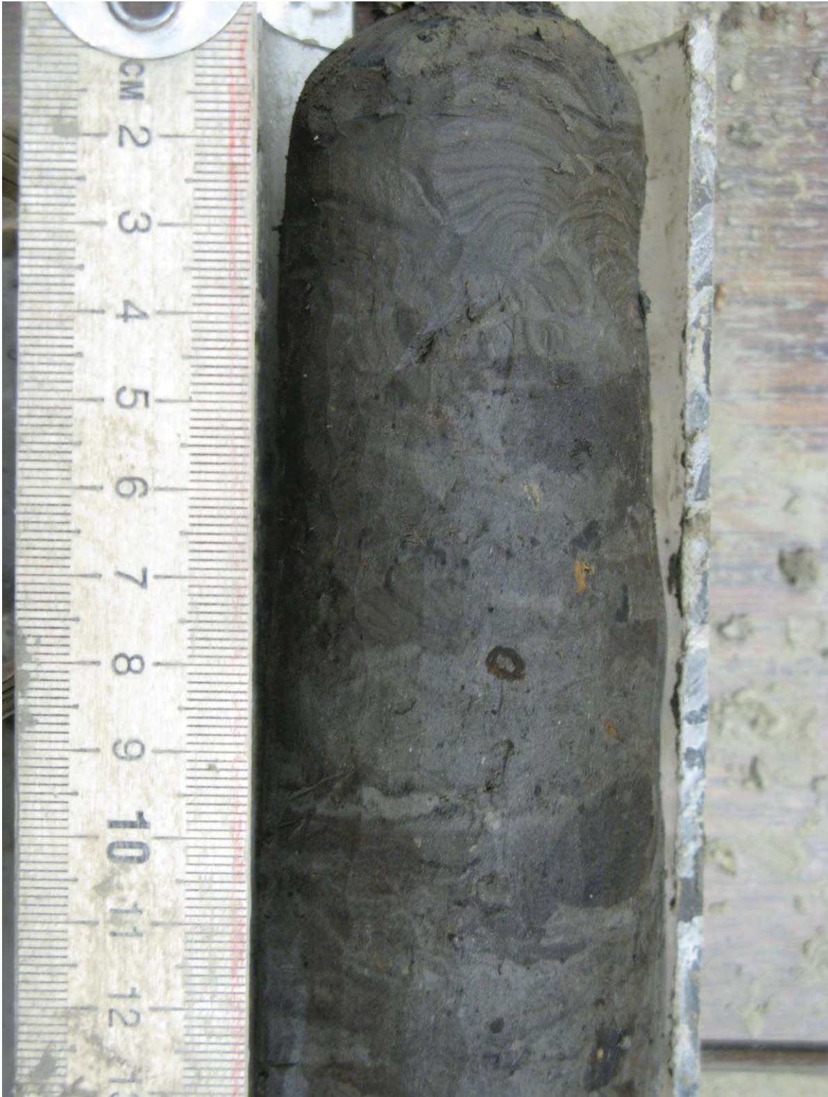
Figure 5.48. Organic silt with porous cryostructure (no visible ice), borehole AUTC-6, depth 2.90-3.03 m, gravimetric moisture content 63%.
