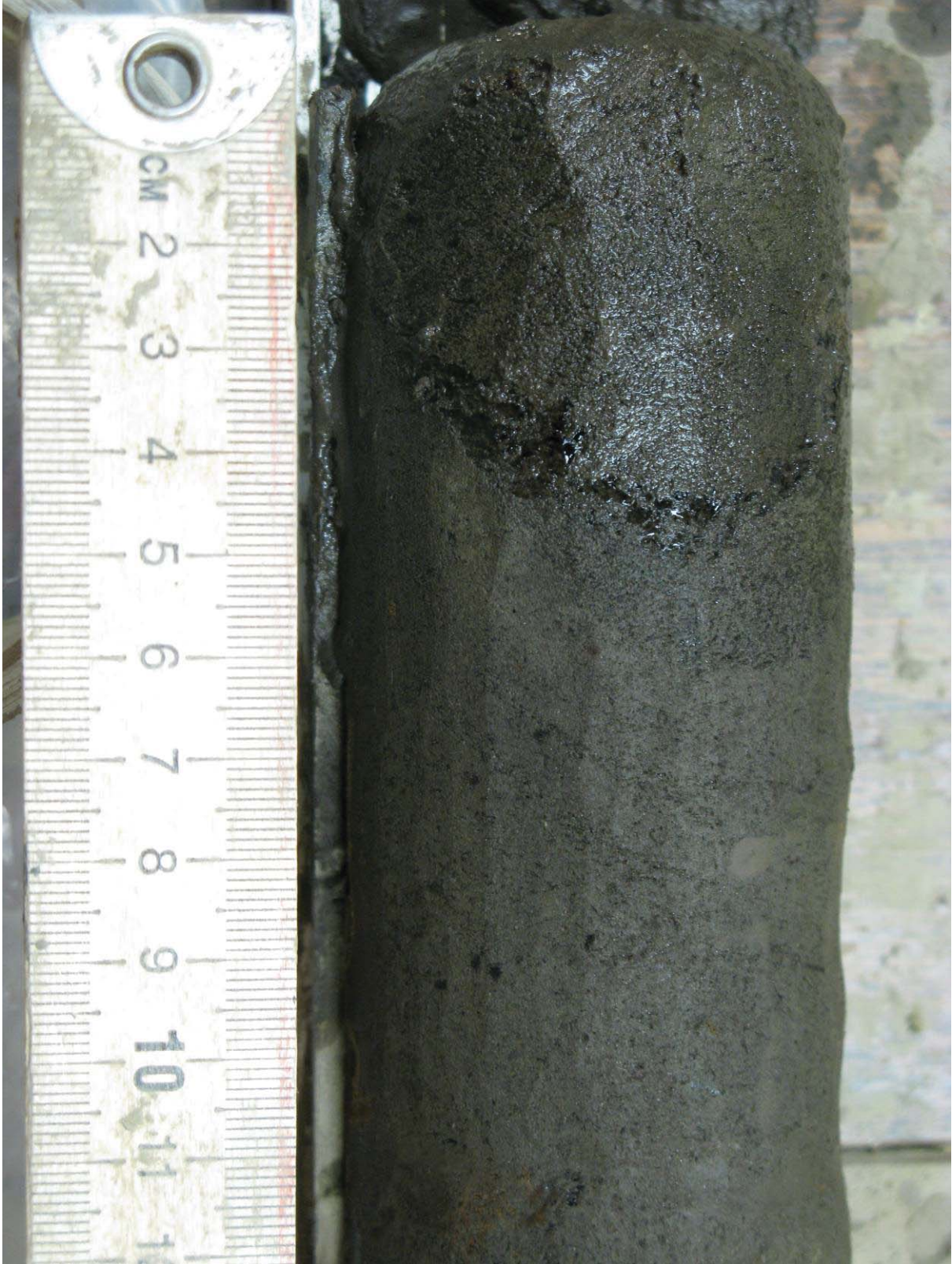
Figure 5.69. Organic silt with organic-matrix – micro-braided cryostructure, borehole AUTC-8, depth 3.60-3.72 m, gravimetric moisture content 93%.
