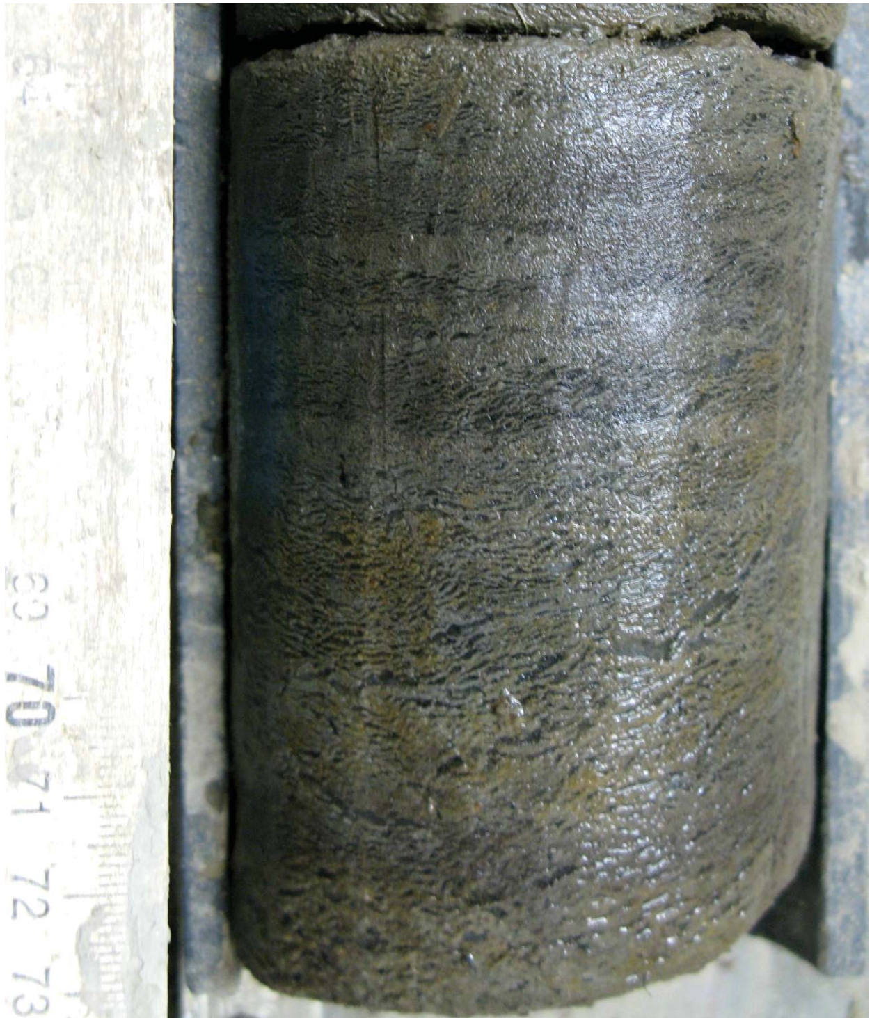
Figure 5.68. Silt with micro-braided – micro-ataxitic cryostructure, borehole AUTC-8, depth 0.64-0.72 m, gravimetric moisture content 182%.
