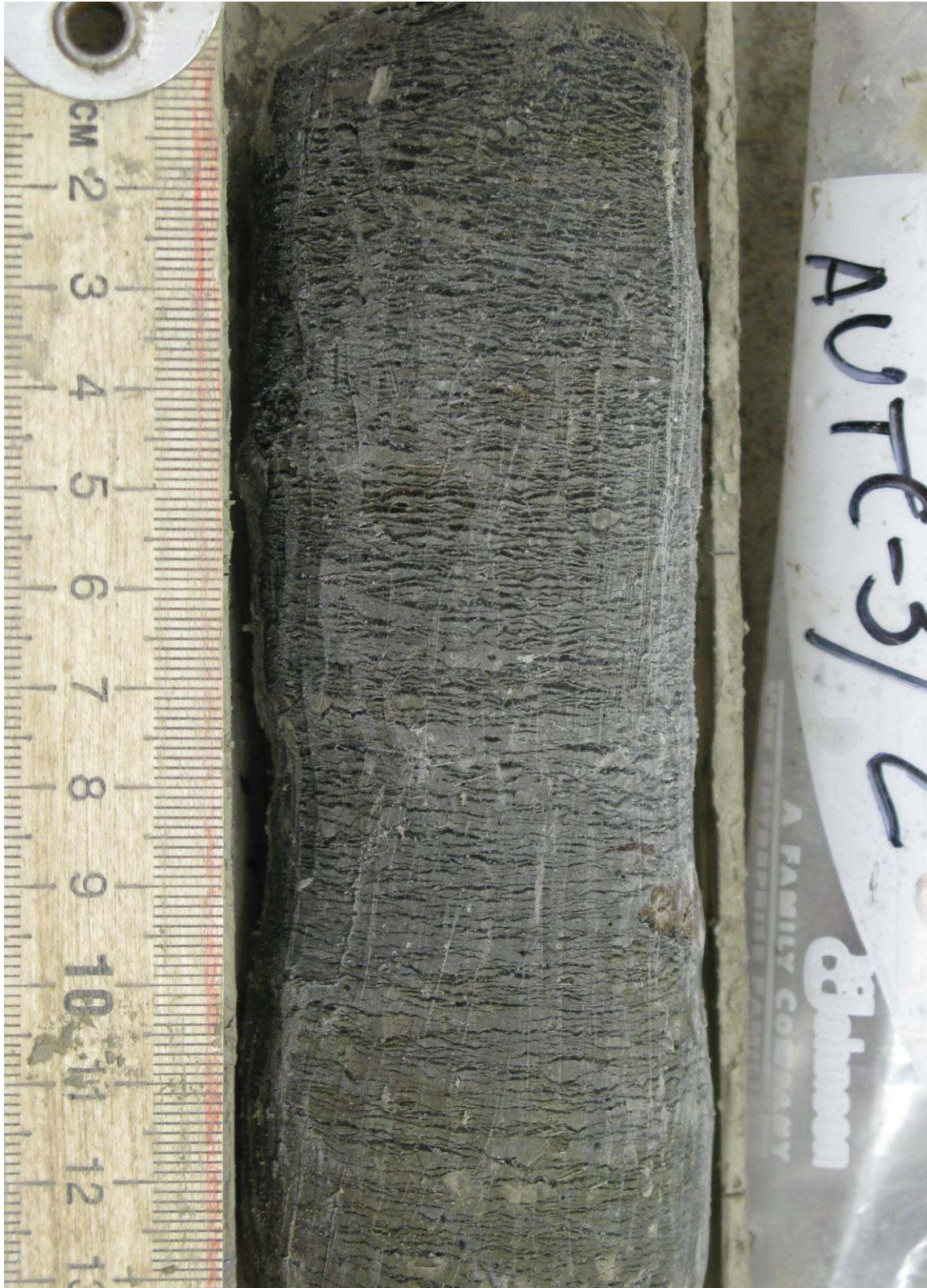
Figure 5.20. Silt with micro-braided – micro-layered cryostructure, borehole AUTC-3, depth 6.0-6.13 m.
