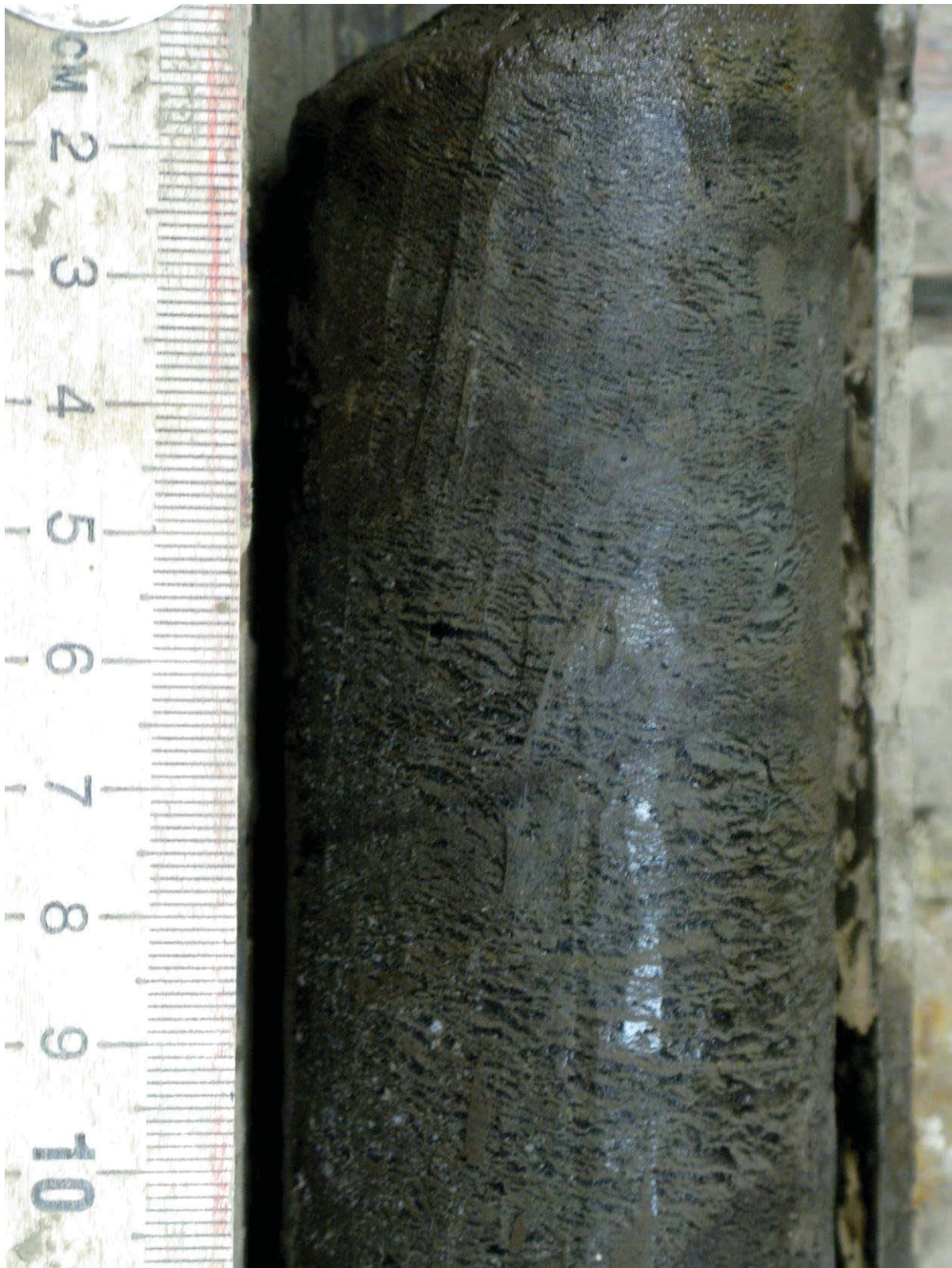
Figure 5.78. Silt with micro-braided – micro-ataxitic cryostructure, borehole AUTC-9, depth 0.91-1.02 m, gravimetric moisture content 160%.
