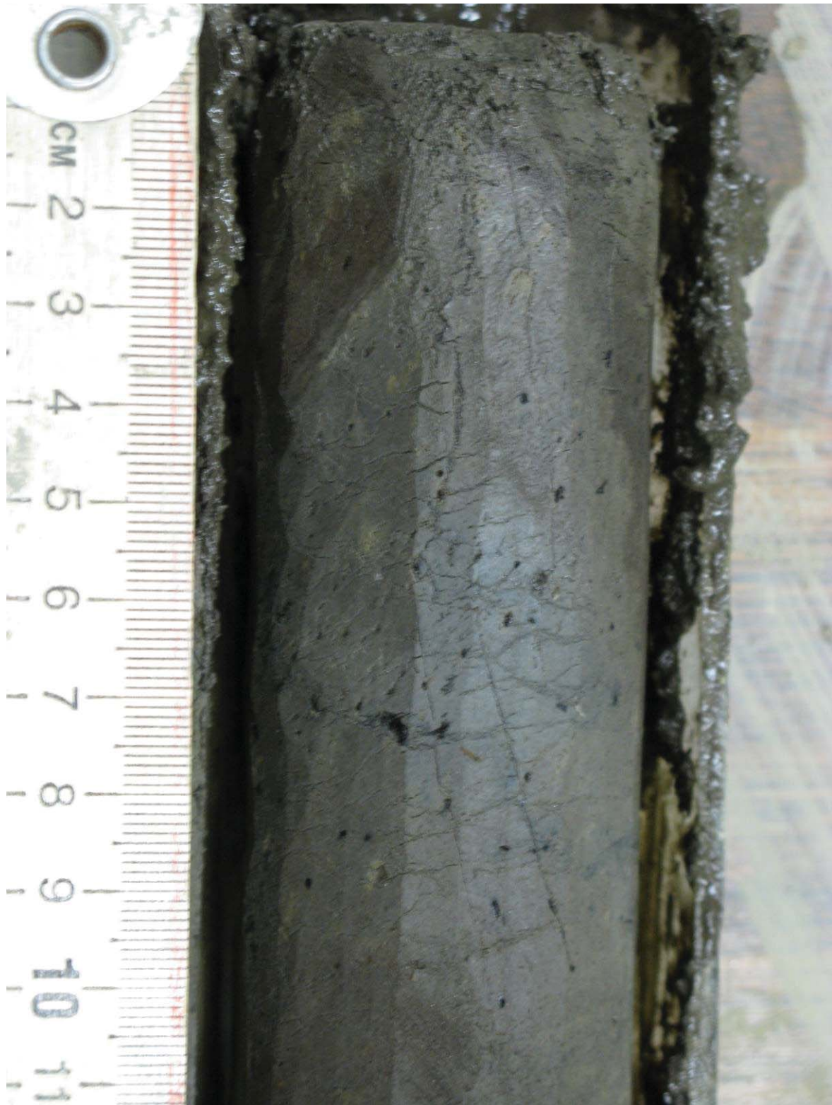
Figure 5.18. Silt with reticulate incomplete cryostructure, borehole AUTC-3, depth 1.65-1.76 m, gravimetric moisture content 68%.
