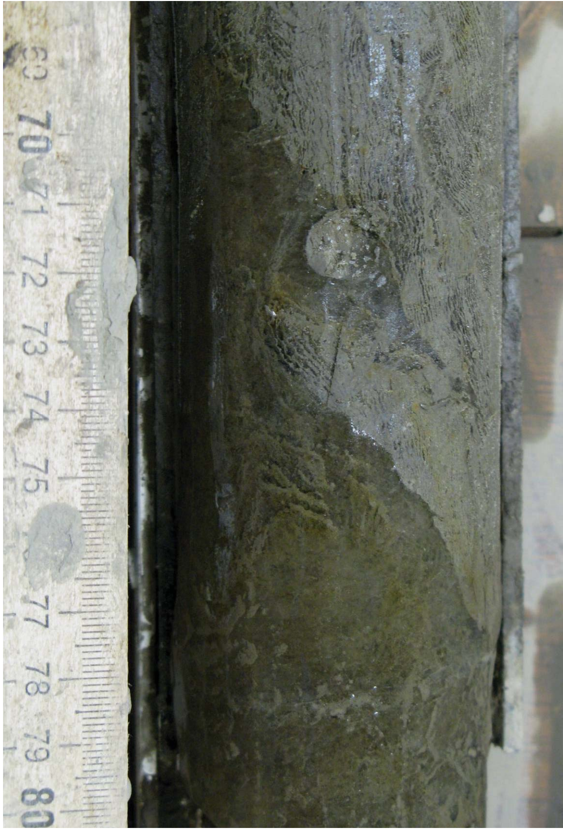
Figure 5.62. Ice-rich silt, boundary with ice wedge, borehole AUTC-7, depth 11.77-11.9 m.
