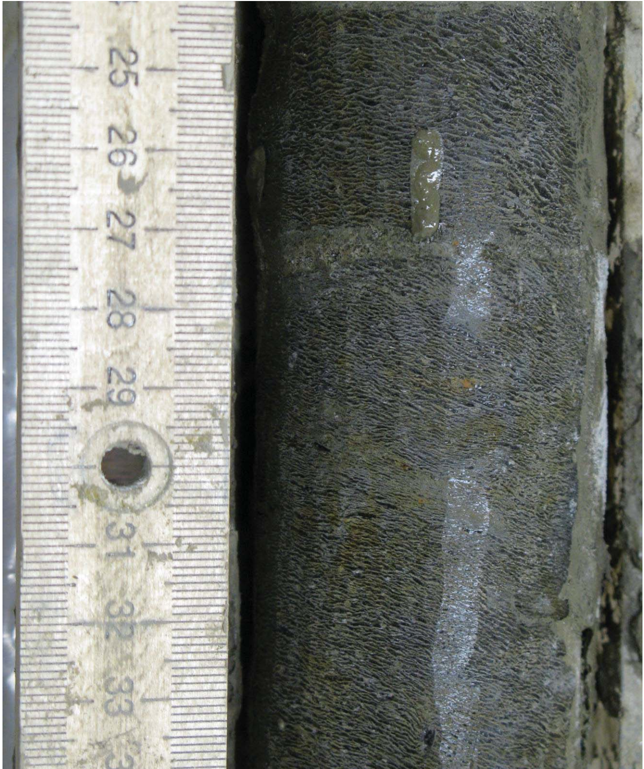
Figure 3.7. Micro-ataxitic and micro-braided cryostructures of syngenetic permafrost (Dalton Highway innovation project area, Interior Alaska).
