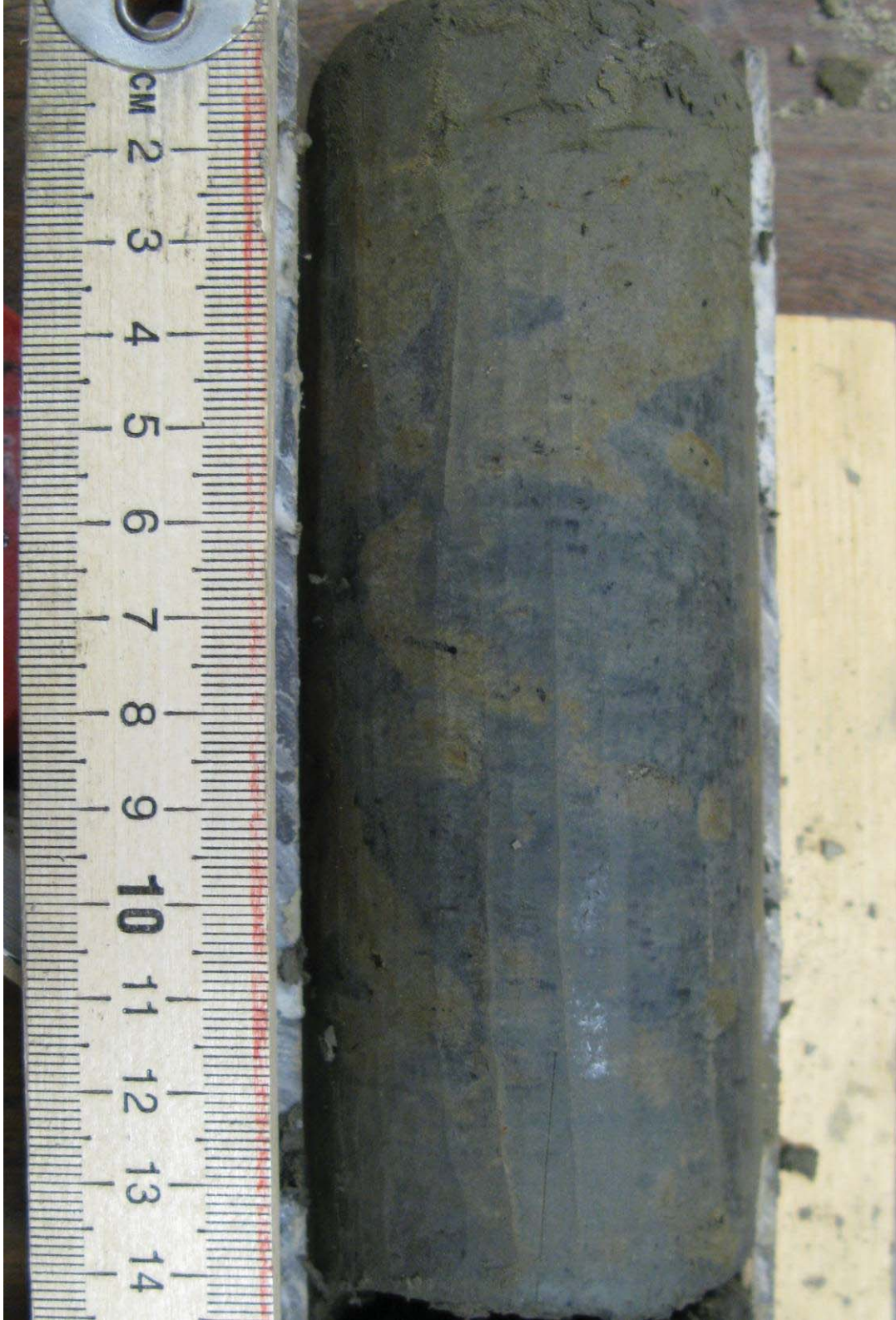
Figure 5.8. Silt with porous cryostructure (no visible ice), borehole AUTC-2, depth 2.80-2.94 m, gravimetric moisture content 46%.
