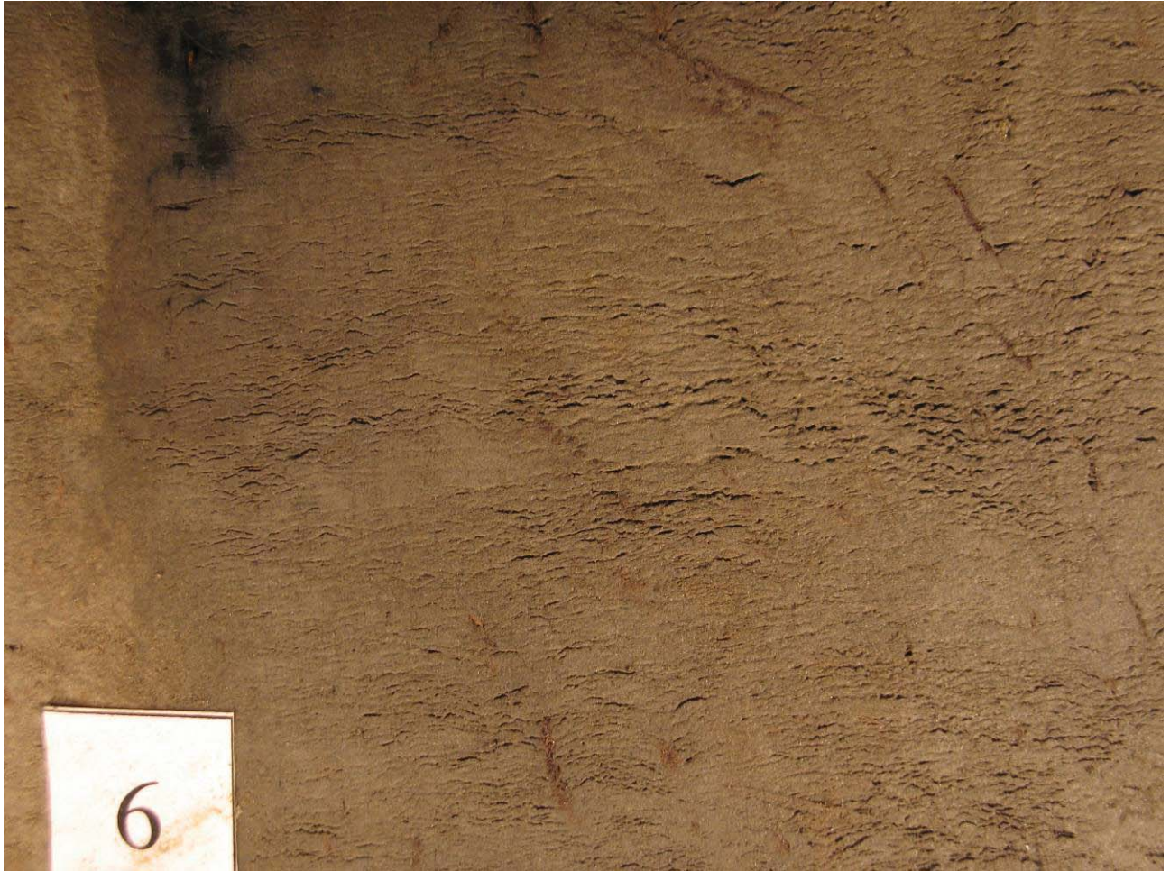
Figure 3.5. Micro-lenticular and latent micro-lenticular cryostructures of syngenetic permafrost, depth 46 ft (14 m), label is 1.25x1.25 cm (CRREL Permafrost tunnel, Fox, Interior Alaska).
