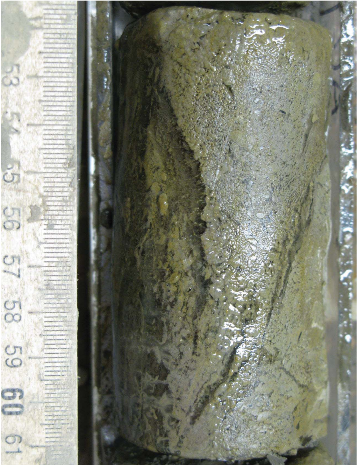
Figure 5.50. Ice-rich silt, boundary with ice wedge, borehole AUTC-6, depth 7.30-7.38 m.
