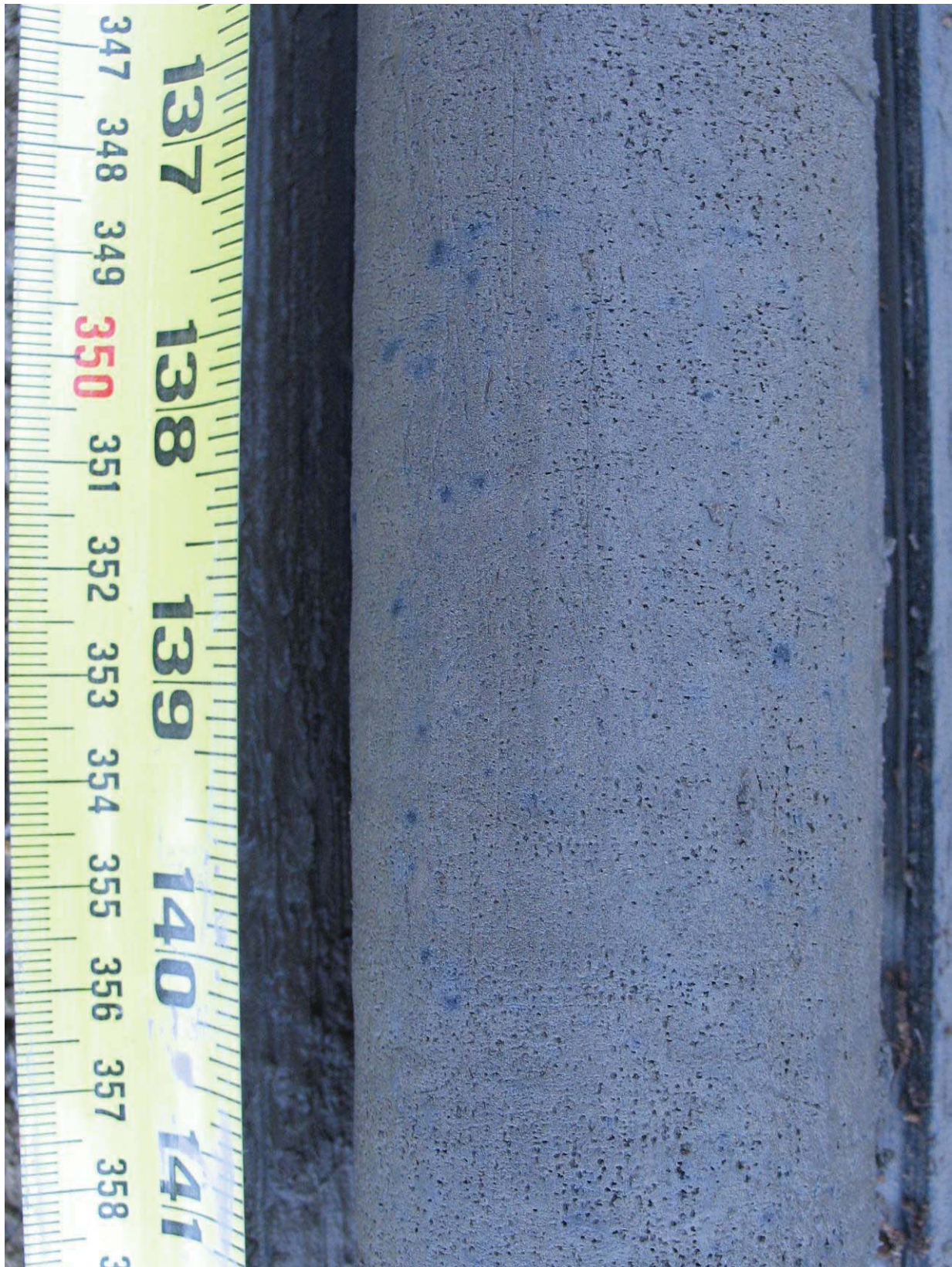
Figure 3.4. Micro-porphyrific cryostructure of syngenetic permafrost (Northern Alaska).
