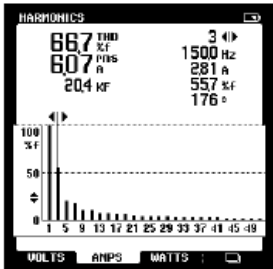
Voltage, current, and power harmonics Up to 51st harmonic Total harmonic distortion (THD) Phase angle of individual harmonics
