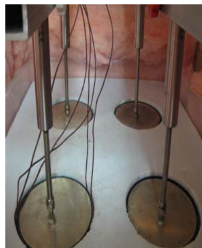
(b) Inside of the frost heave cell
