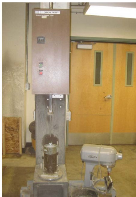
Figure 3.4 Automatic mechanical compactor
