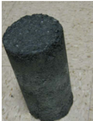
Figure 3.12 Compacted aggregate base course specimen
