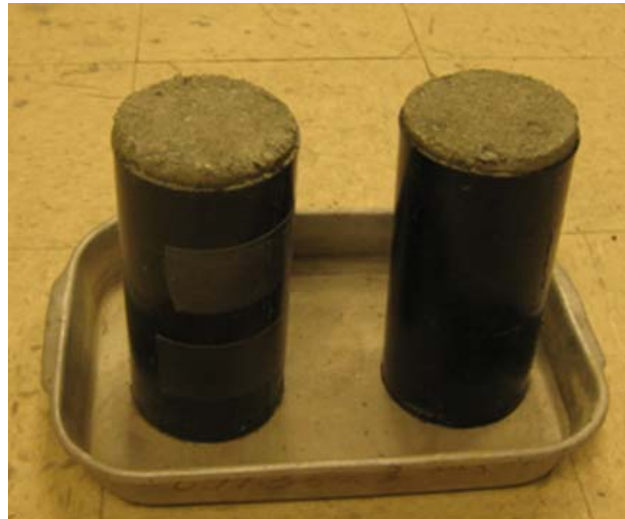
Figure 3.20 Specimens after frost heave test
