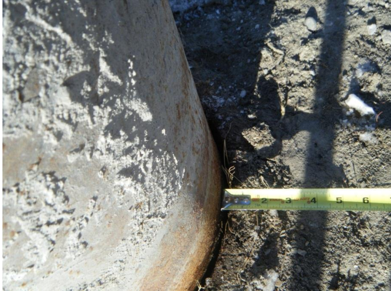
Figure 2.31: At 207 kips, unloaded plastically deformed soil gap in front of the test pile.
