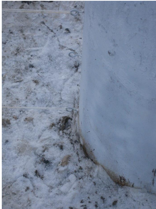
Figure 2.26: Soil crack at 150 kips, January test.
