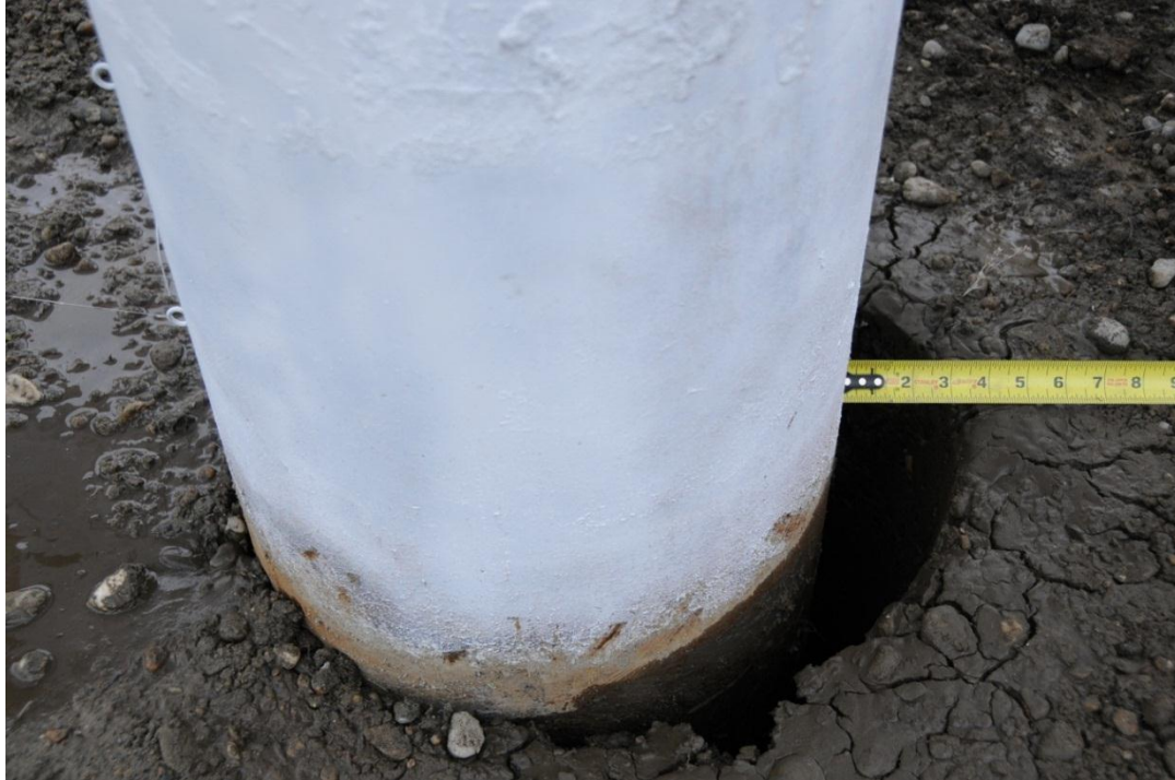
Figure 2.22: Plastically deformed soil; test pile after final loading and unloading.
