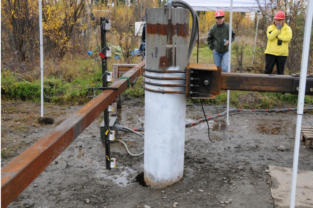
Figure 2.20: Test pile at final September load increment.
