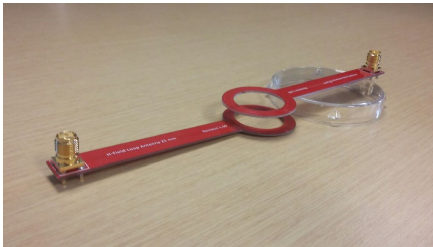
Figure C-3. PCB level design of the EC testing, also used for SE measurement based on the IEEE standard.
