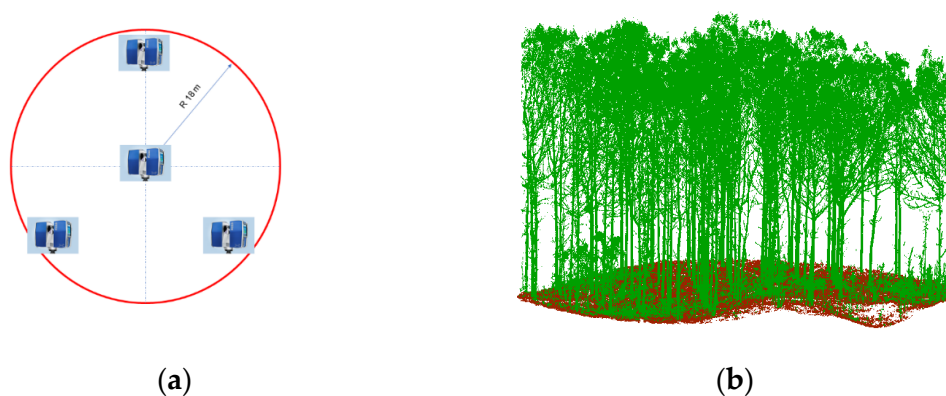
Figure 2. Reference plots geometry and Terrestrial Laser Scanning (TLS) derived point cloud. (a) Circular reference plots for TLS field work showing the four scans pattern; (b) semi-automatically segmented TLS point cloud showing ground (brown) and vegetation (green) classified points. Case study: Reference plot located in El Tecal plantation.
