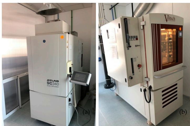
Figure 1. Weathering chambers used in the corrosive tests: (a) SC 340 MH; (b) VCC 3 0034 Vötsch.
