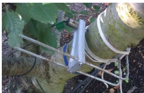
Picture 8. LVDT sensor installed in a tree branch measuring its diameter variations.
