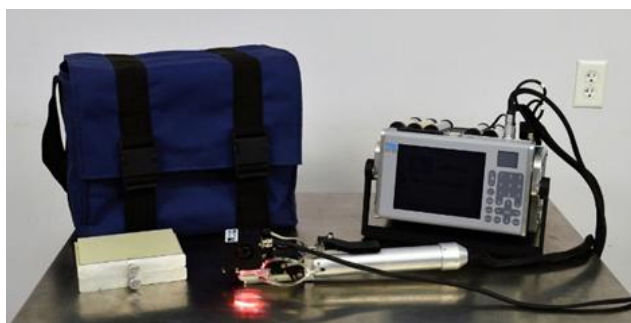
Picture 7. CIRAS-2 portable photosynthesis system.
