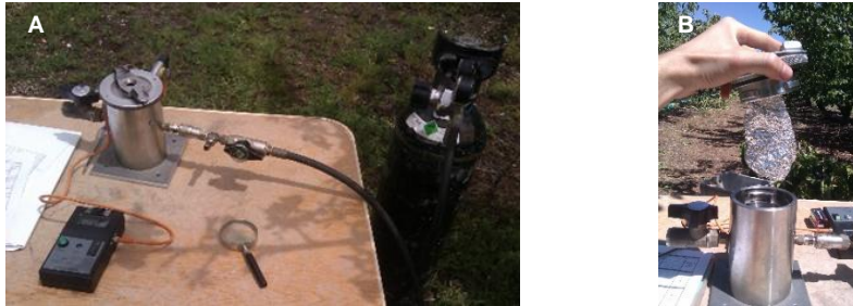
Picture 6. Scholander pressure chamber (A) and covered leaf ready to be measured (B).
