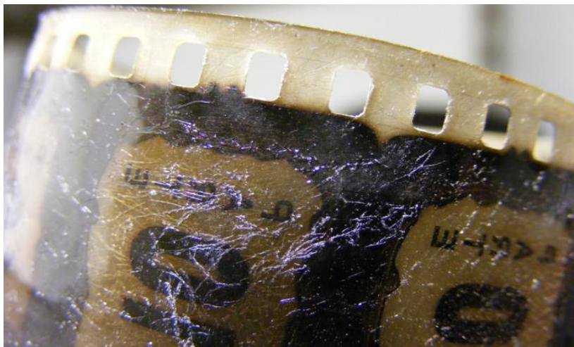
Figure 11 - Detail of cracks on the emulsion layer and plasticizer deposits on the film surface © Teréz Somfai
