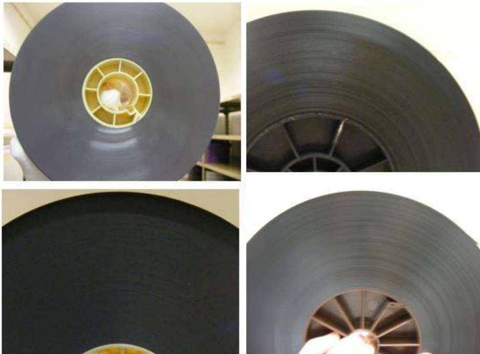
Figure 31 - Light transmission test: MAG on PET support © ANIM/Credits: Teréz Somfai
