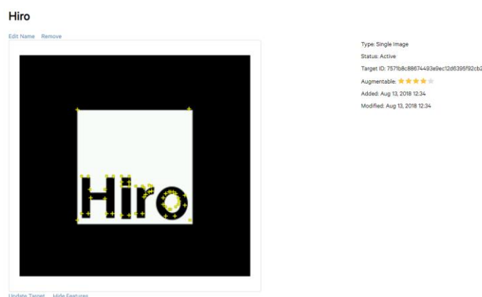
Figure 27 Feature points from Hiro Image Target
