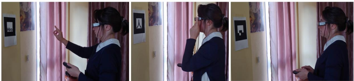
Figure 48 Interaction Methods with a) gestures b) head movement and on-device interaction c) and with the smart glasses controller
