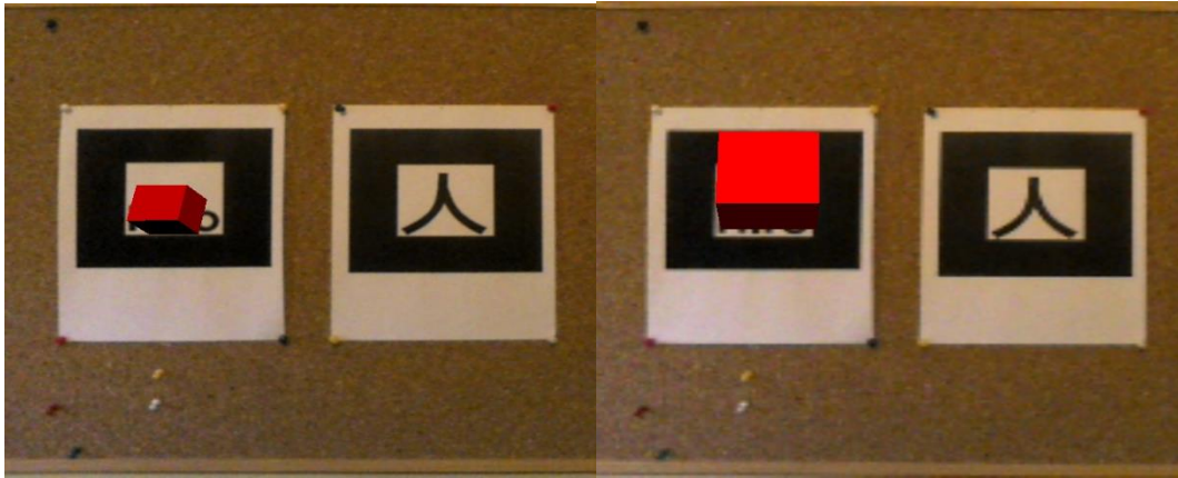
Figure 31 Tracking with NyARUnityNftSystem (left) Tracking with NyARUnityMarkerSystem (right)
