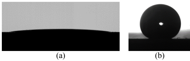
Fig. 4. Typical photographs of distilled water droplets on the surface immediately after texturing (a) and after six hours of heating (b).
