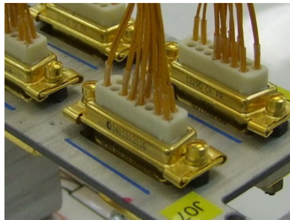
Fig. 3. Crimping is used for ESA-made connectors
