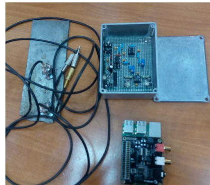
Fig. 3. Vibration signals receiving unit on Raspberry Pi 3B+
