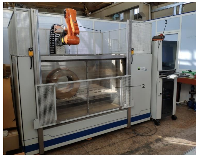
Fig. 3. The current experimental facility (1 – robotic manipulator, 2 – immersion bath, 3 – control cabinet)
