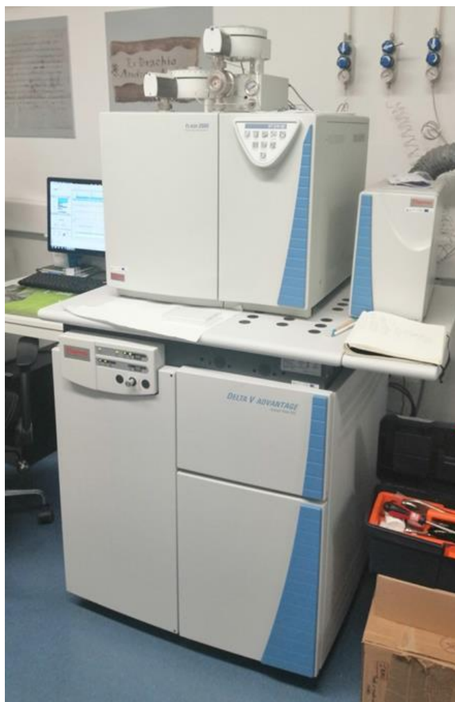
Figure 19. EA-IRMS equipment used for the analyses of carbon and nitrogen stable isotopes of this study in HECULES Laboratory.
