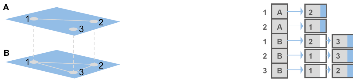
Figure 2.3: A multiplex graph and its correspondent adjacency list. A list for each node instance.
