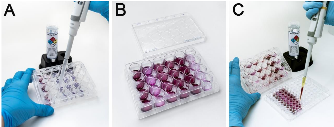
Figure 10. Use DMSO to solubilize the formazan crystals (A), this solubilization originates a purple solution (B) and then transfer the obtained solution from each well to a 96-well plate (C).
