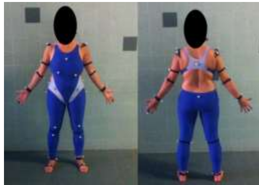
Figure 3.1 – Reflective body marker setup model with 48 body markers.
