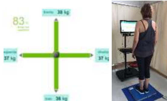
Figure 6.4 - Monitor picture of physio sensing platform for good feedback as be in balance and a subject collect moment.
