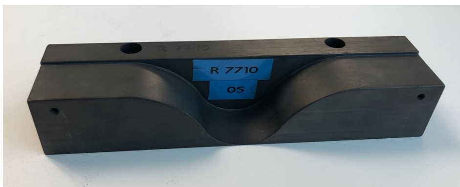
Figure 2.1. A CT shaped filter. Courtesy of Sebastian Faby (Siemens Healthcare, Forchheim, Germany).
