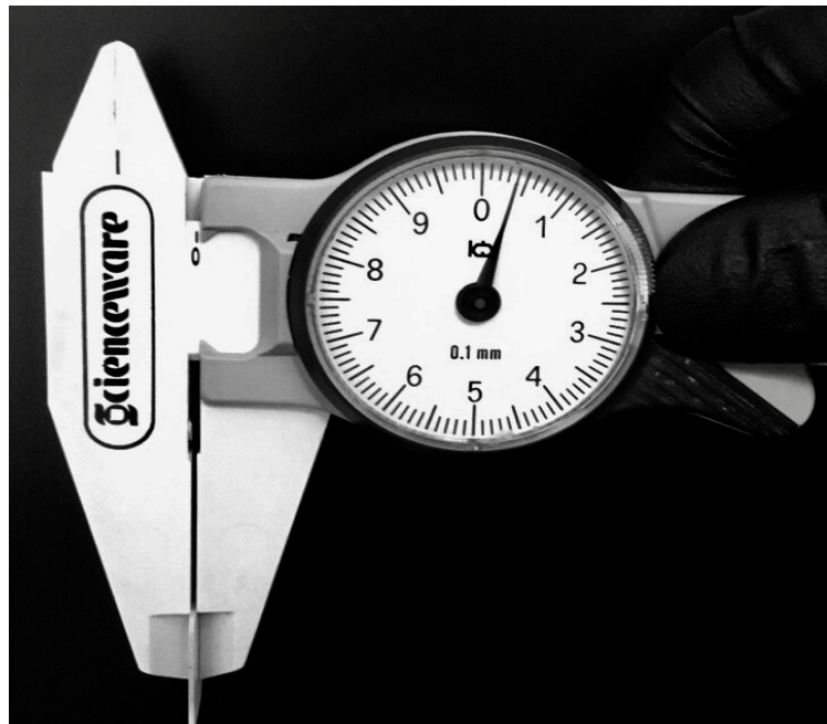
Figure 4. Caliper to Measure the Ceramic Thickness of 0.4mm
