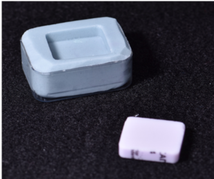
Figure 8. E.max Slice used to make a Custom-made mold to Fabricate Slice-Shaped Composite
