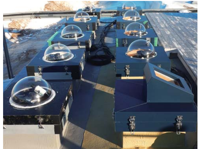
Auroral optical observation instruments at Syowa Station.
