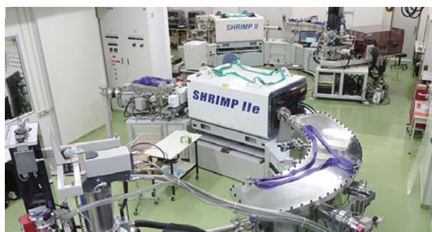
Sensitive high resolution ion microprobe (SHRIMP) for age dating of minerals.
