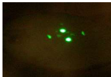
A field emission pattern from after treated Sc-oxide/W emitter.
