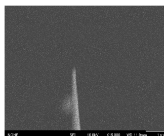
The radius of the Sc-oxide/W emitter The radius r=0.167 \mu\text{m}
