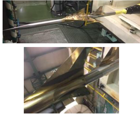
Fig. 9. A wing tunnel test model installed in the transonic wind tunnel.
