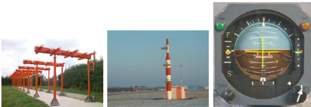
Figure 1.5 Localizer aerial, glide slope installations and ILS indicator [4].
